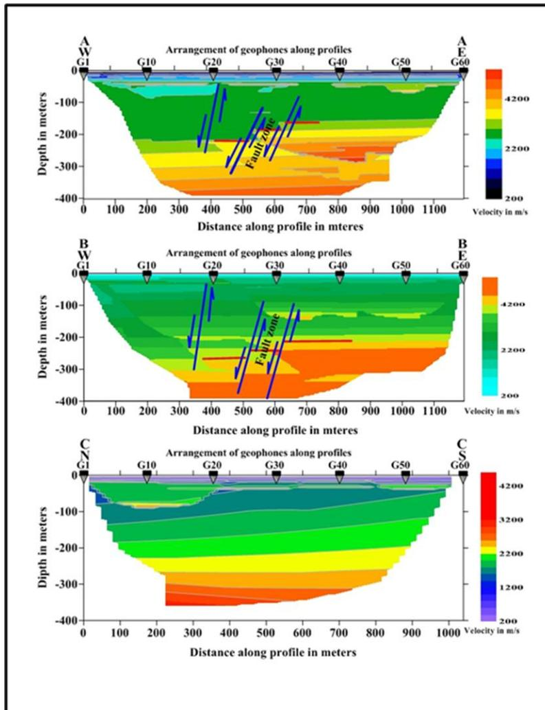
Fig (3): Seismic velocity field sections along AA, BB, and CC profiles.
