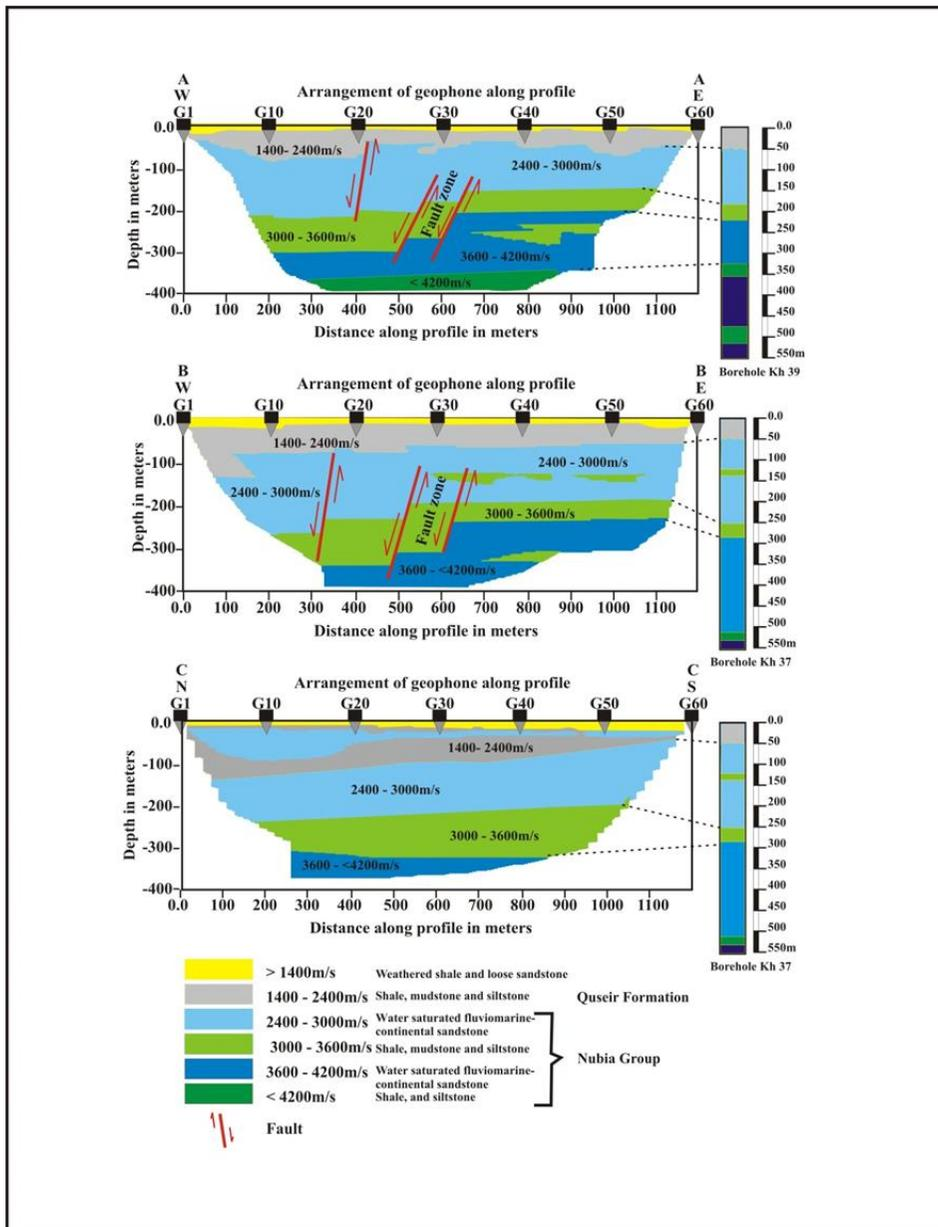
Fig (4): Geoseismic cross section along AA, BB, and CC profiles.
