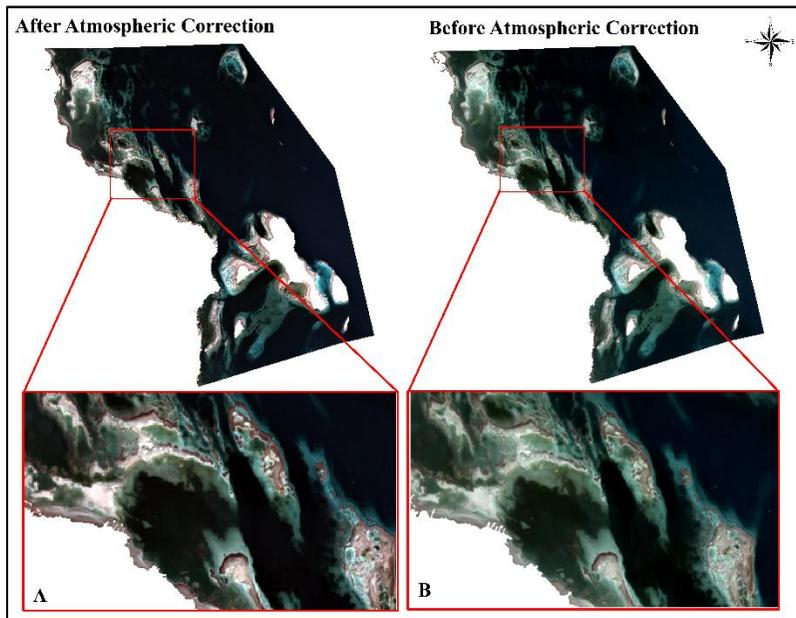
**Figure 2:** Landsat image before and after the atmospheric correction; (A) and (B) are the zoomed areas near Al Ahiaa district coral reef after and before the atmospheric correction.
