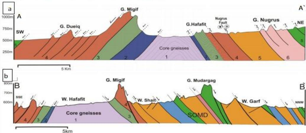
Fig.3: (a) A-A' and (b) B-B' schematic cross-sections to illustrate the structural setting in two profiles crossing the structural map in fig.2.
