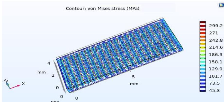
**Figure (2) Distribution of Von-Mises stress on composite sheet.**
