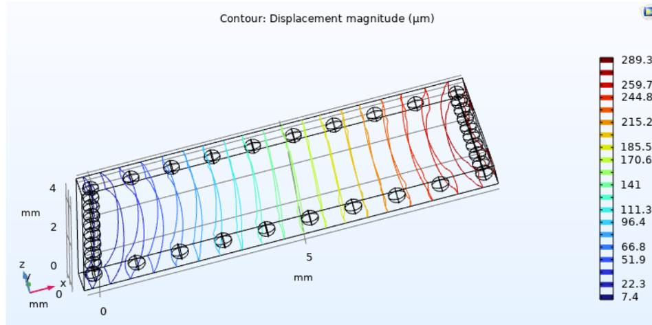
**Figure (7) contour diagram of a new design of composite sheet: edge reinforcing composite sheet.**
