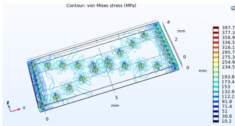
**Figure (8) Von Mises stress contour diagram for a new design of composite sheet (diagonal reinforcing composite sheet).**
