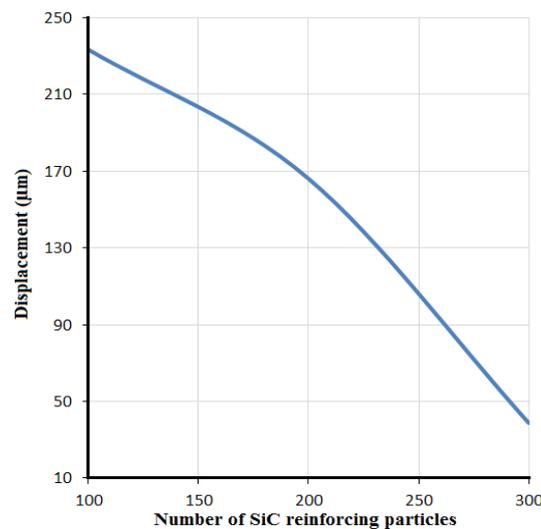
**Figure (5) Impact of SiC reinforcing particles quantity on displacement of composite sheet.**
