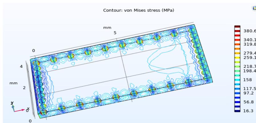
**Figure (6) Von Mises stress contour diagram for a new design of composite sheet (edge reinforcing composite sheet).**
