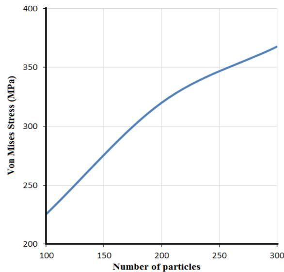
**Figure (4) Impact of SiC reinforcing particles quantity on Von Mises stress.**
