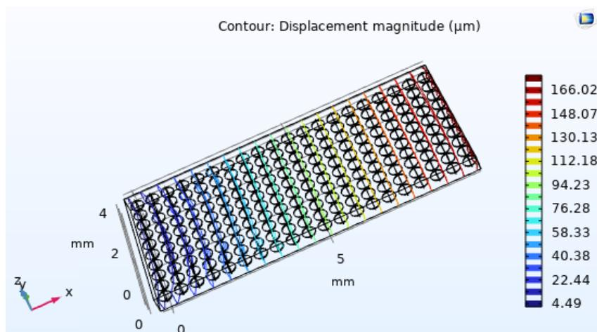
**Figure (3) contour diagram of displacement 27% SiC epoxy composite sheet.**
