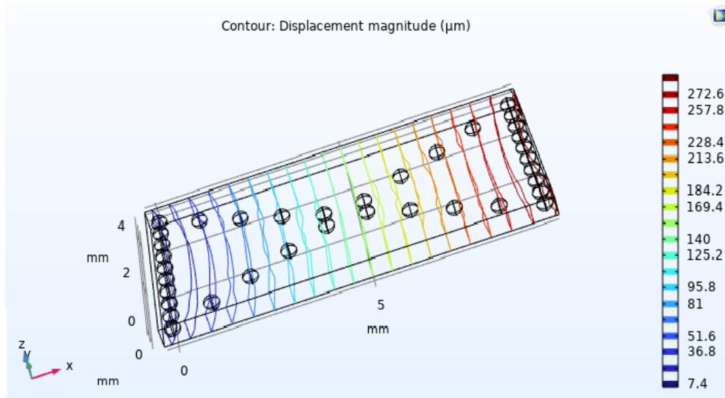
**Figure (9) contour diagram of a new design of composite sheet: diagonal reinforcing composite sheet.**
