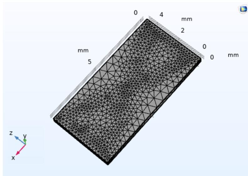
**Fig.1 Meshing net for composite sheet.**
