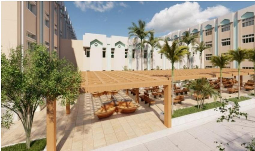
Figure 20: Shows the presence of wooden pergolas to reduce heat islands and increase the shaded area.
