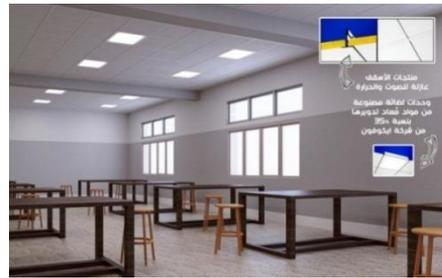
Figure 36: Using suspended ceilings from recycled materials, which are sound-absorbing and heat-insulating.
