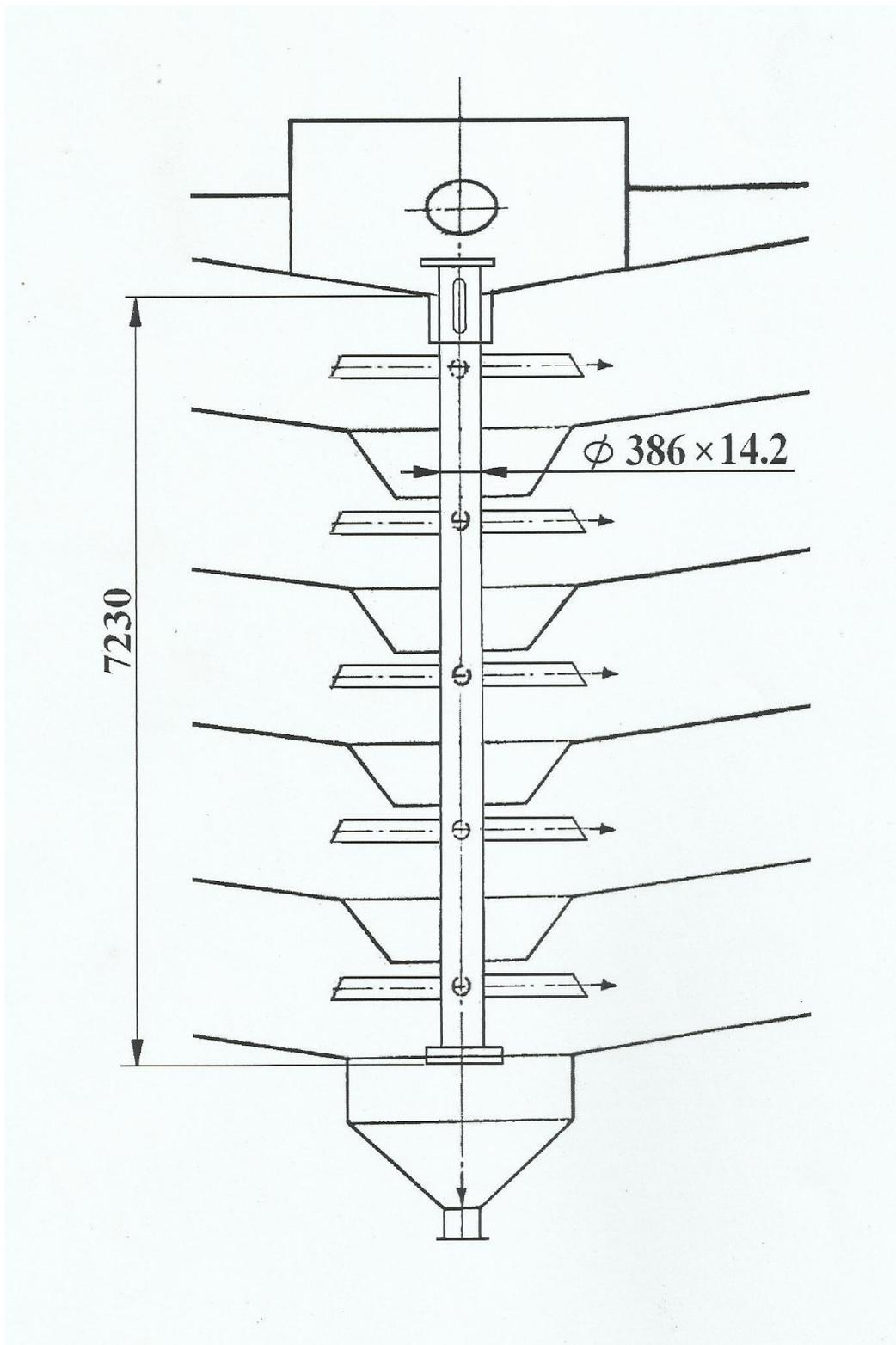
**Fig. 3. Clarifier Central Tube Structural Form The above two figures was done by the Armant Engineering Drawing Office**
