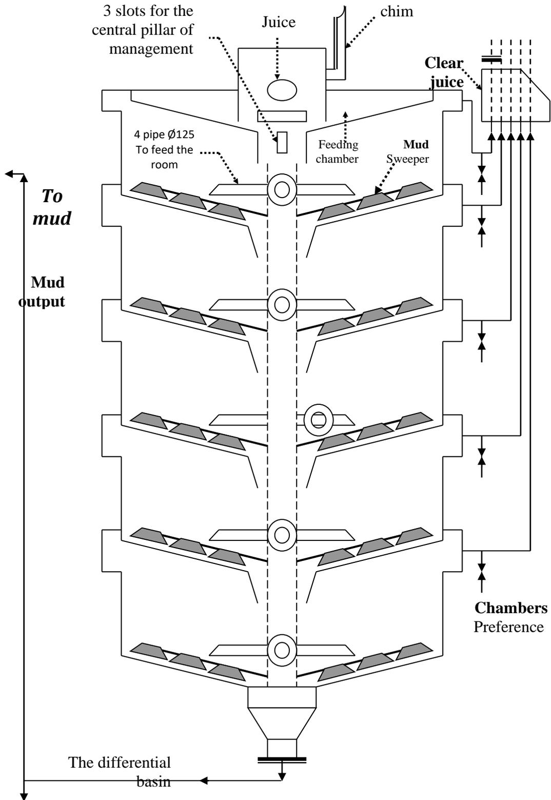
**Fig. 2. Clarifier Structural Form**
