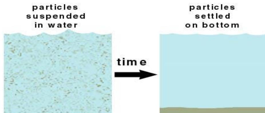
**Fig 4 Sedimentation process<sup>(9)</sup> .**
