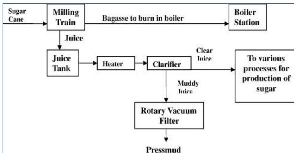
Fig. 1. A schematic diagram of formation of pressmud waste in sugar mill.
