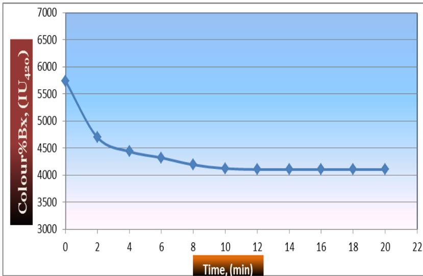
**Figure (8): Effect of contact time on colour removal from raw cane juice by modified bentonite at constant pH and temperature.**
