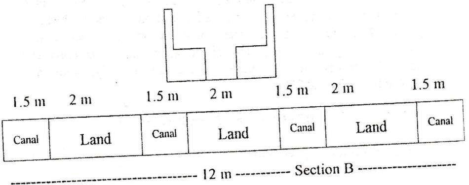
Fig. (2): The construction of the canals for field canal experiment.
