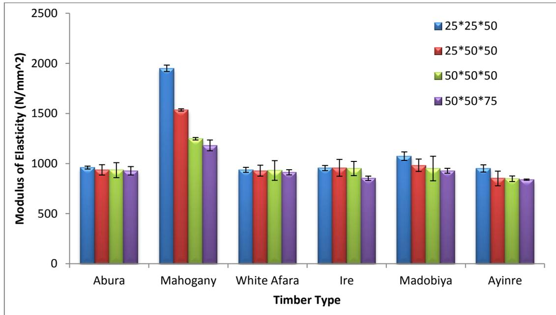
Figure 7: Elastic Modulus for Varying Section of the Timber Samples
