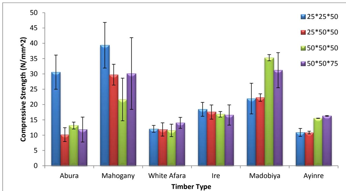
Figure 6: Compressive Strength for Varying Section of the Timber Samples
