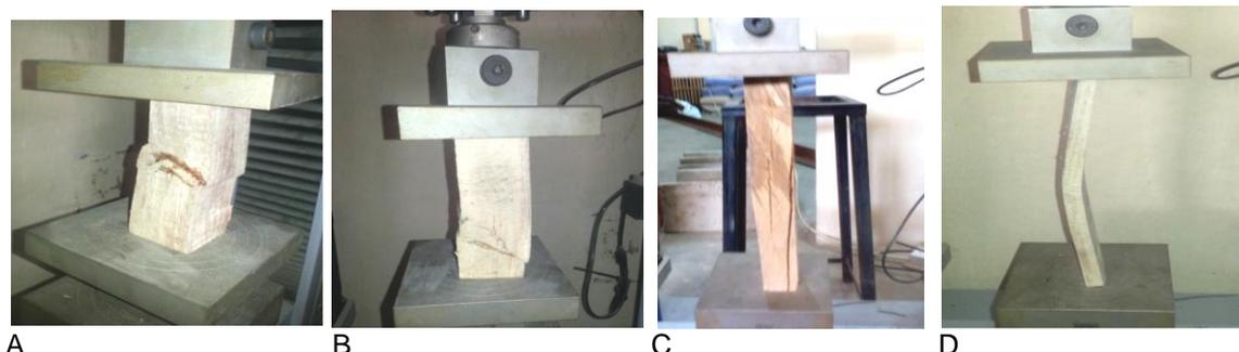
Figure 6: Typical shearing (A), crushing (B), splitting (C), and buckling (D) failure modes of timber samples oriented parallel to grain and under compression.
