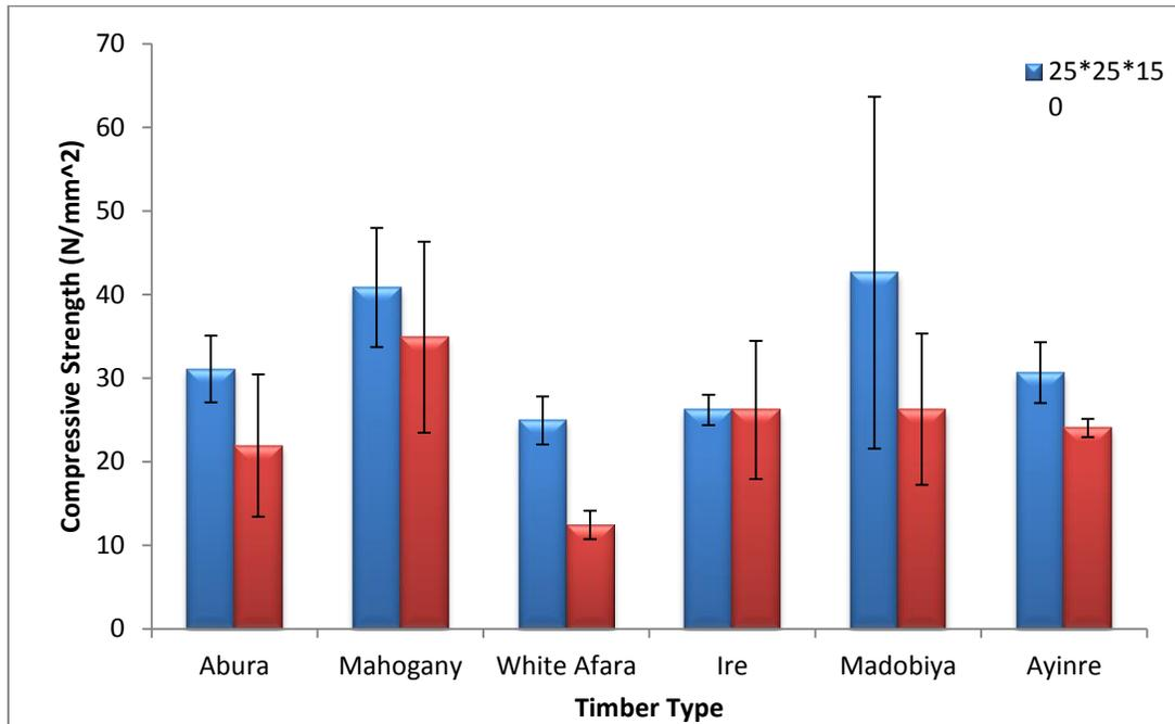
Figure 3: Compressive Strength Results for Varying Sections of the Timber Species
