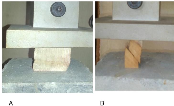
Figure 7: Typical crushing (A) and shearing (B) failure modes of timber samples under compression force perpendicular to grain.
