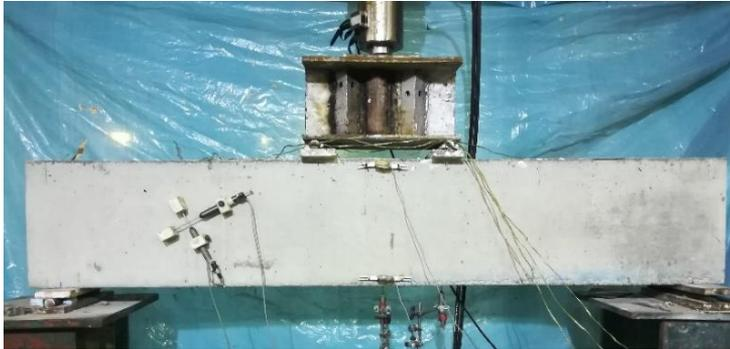
Fig. 5 Test setup and instrumentation
