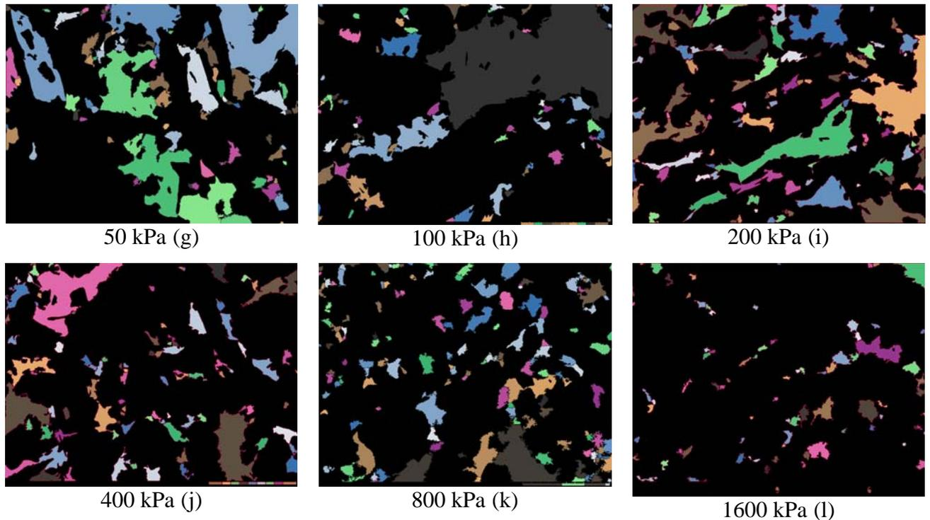
**Fig.6 PCAS analyzed image of soft clay under different pressures**
