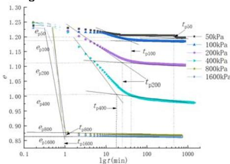
**Fig. 4 Curve of  $e \sim \lg t$  of the soft soil on different consolidation stresses**
