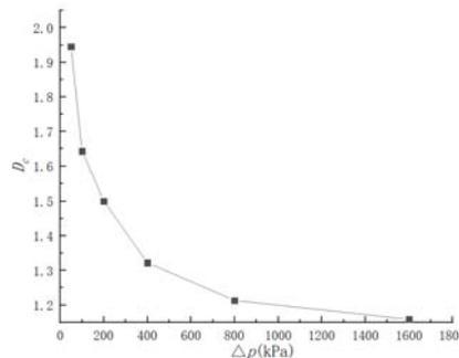
**Fig.8 Variations of pore porosity fractal dimension under different pressures**
