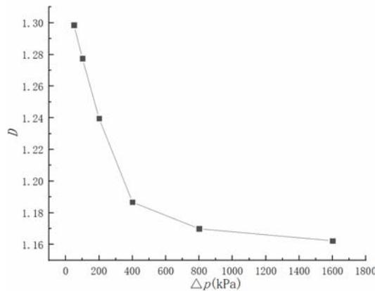
**Fig.10 Variation curve of pore fractal dimension under different pressure**
