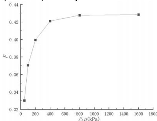
Fig.10 Variation curve of average shape coefficient under different pressure
