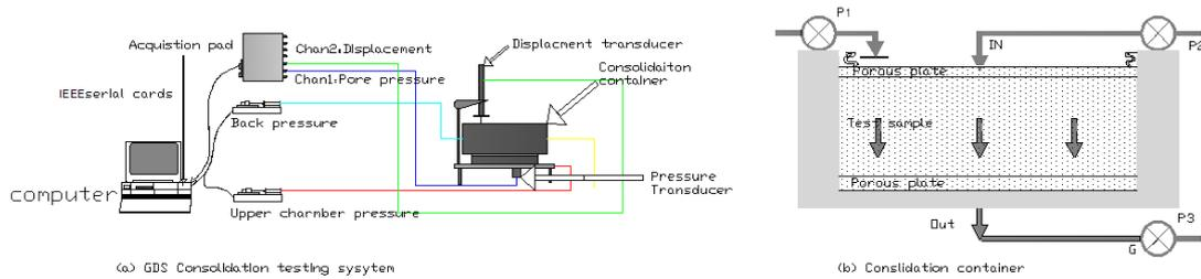
**Fig. 2 GDS Advanced Consolidation Testing System**
