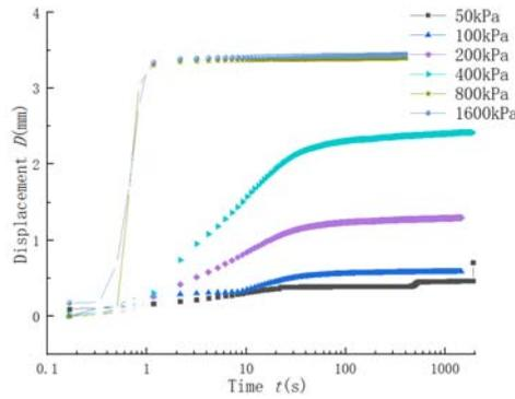
**Fig. 3 Curve of time-displacement under different consolidation stresses**
