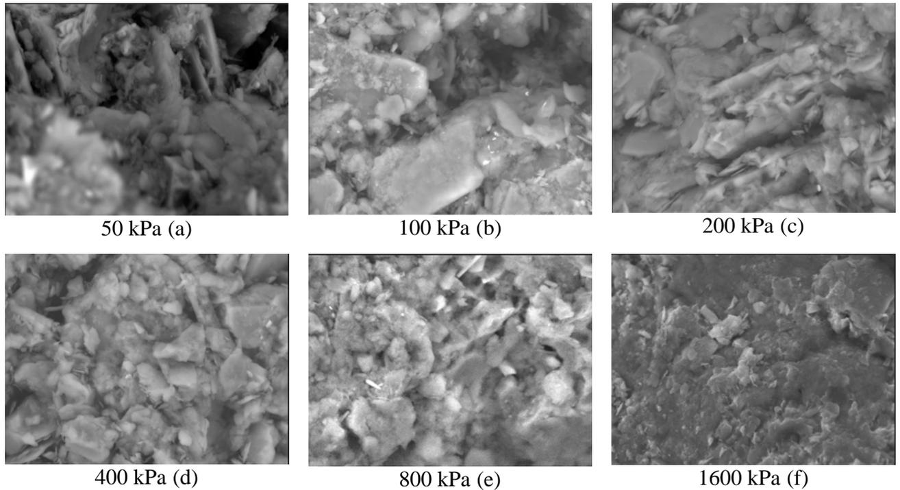
**Fig.5 SEM image of soft clay under different pressures**
