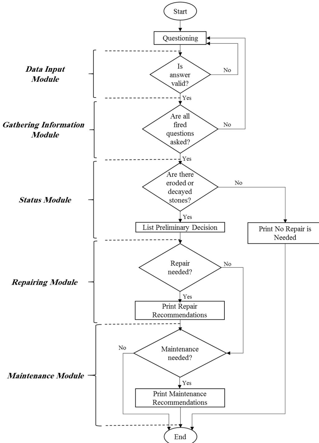
Fig. 1: ES\_HXWall system flowchart
