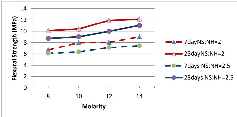
Figure 6: Effect of concentration of sodium hydroxide solution
