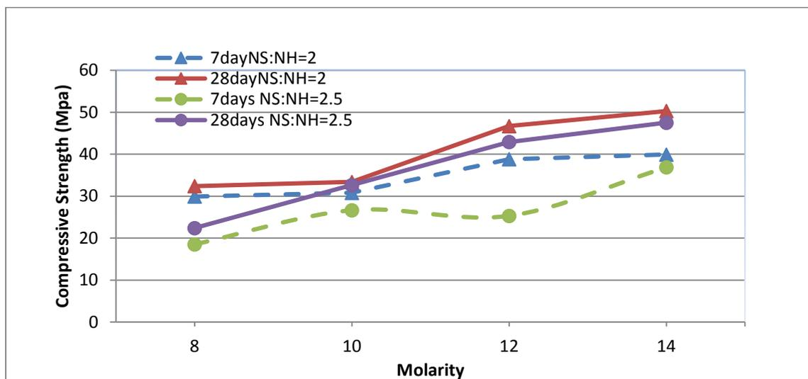
**Figure1: Effect of concentration of sodium hydroxide solution**
