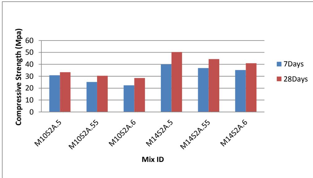
Figure 2: Effect of ratio of activator to fly ash
