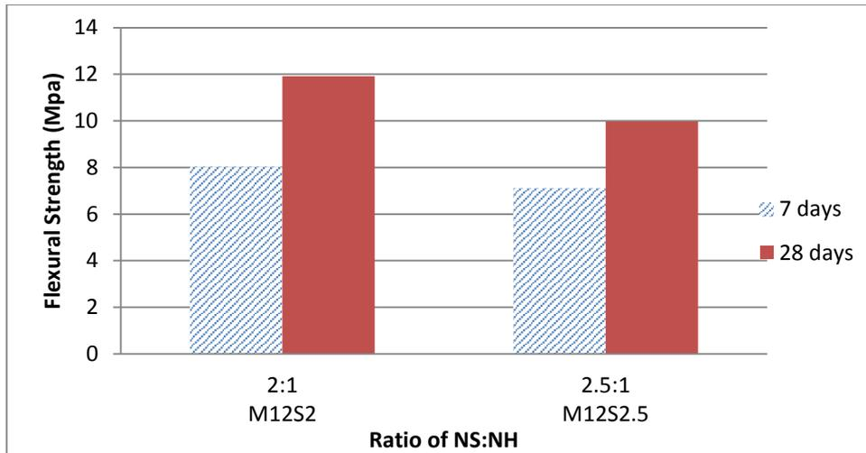
**Figure 8: Effect of varying ratio of sodium silicate to Sodium hydroxide solution**
