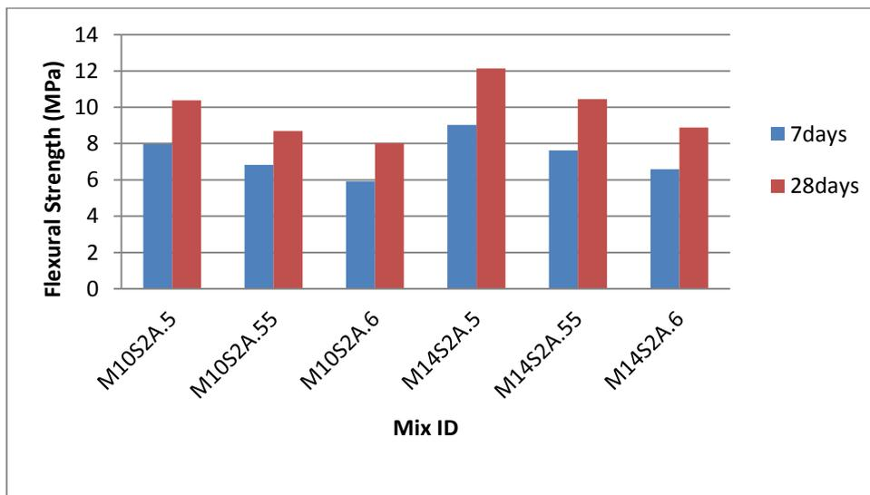
Figure7: Effect of ratio of activator to fly ash
