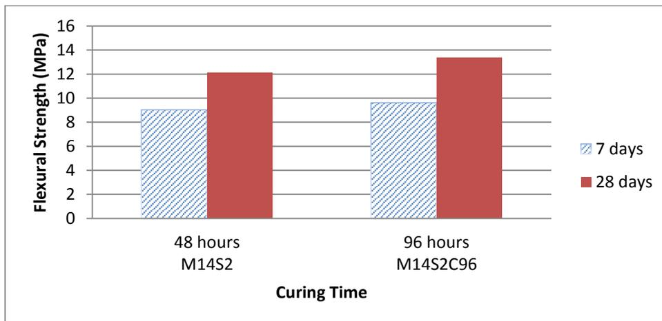
**Figure 9 : Effect of varying the curing time**
