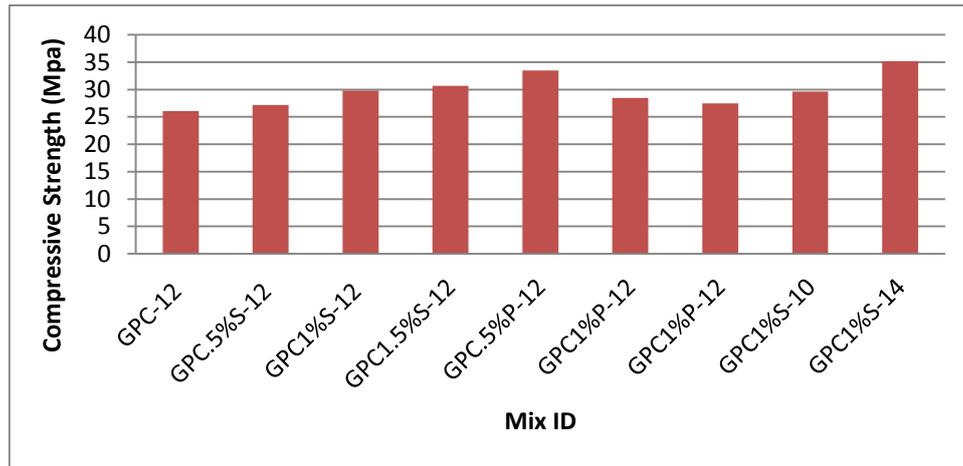
Figure 11: Compressive strength of GPC mixes at 28 days
