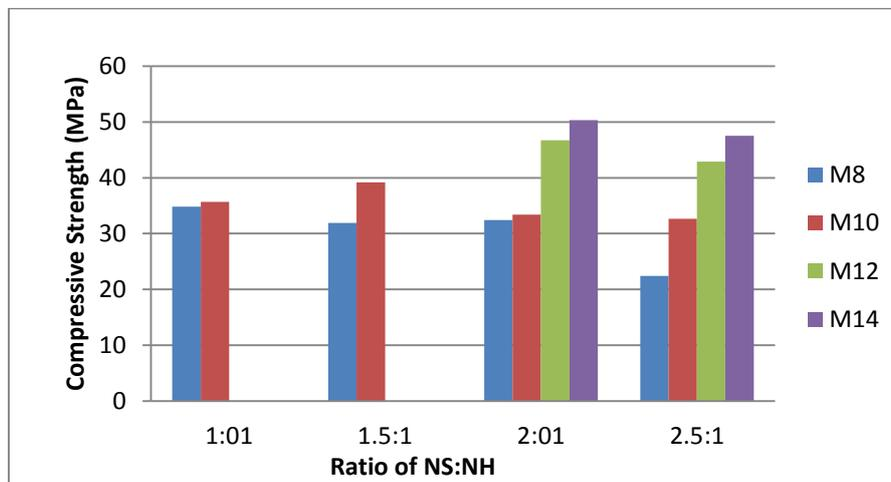
Figure 3: Effect of varying ratio of Sodium Silicate to sodium hydroxide solution
