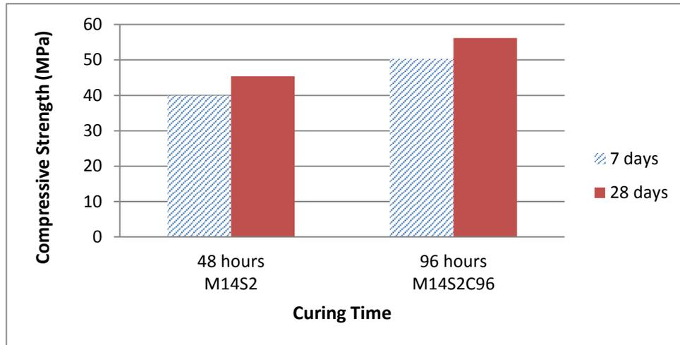
Figure 4 : Effect of varying the curing time
