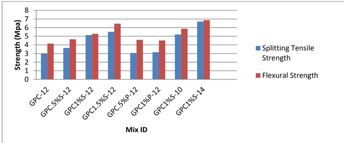
Figure 12: Splitting tensile and flexural strengths of GPC mixes at 28 days
