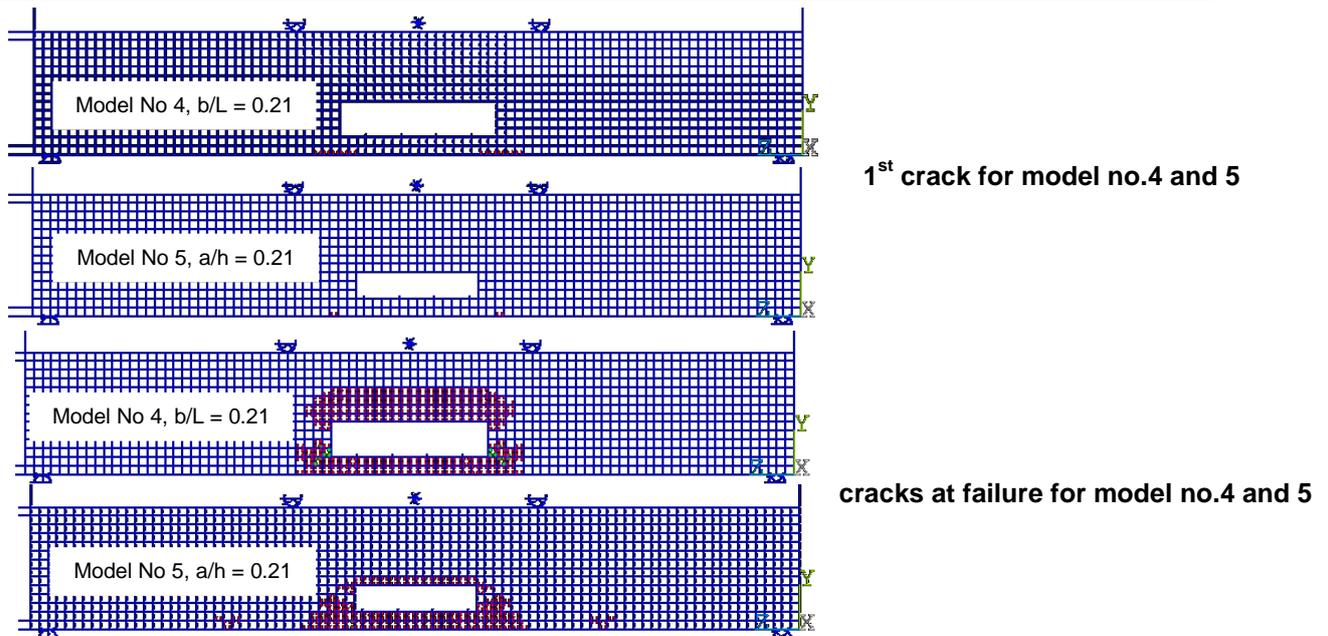
Fig. 16 Patterns of 1<sup>st</sup> crack and cracks at failure for RC beam model no.4 and 5
