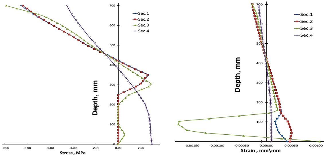
Fig. 9 Distribution of normal stress and normal strain for the selected sections in control RC beam
