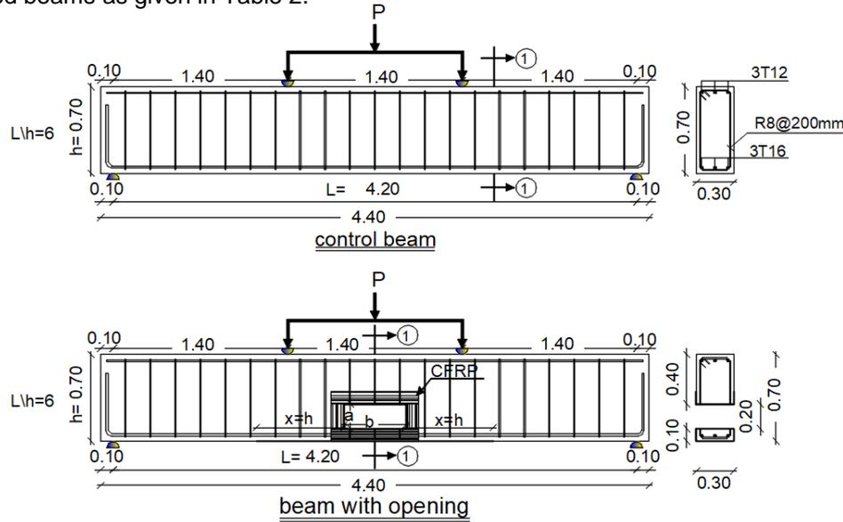
Fig. 5 Schemes for control RC beam and RC beam with opening
