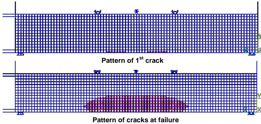
Fig. 10 Patterns of 1<sup>st</sup> crack and the cracks at failure for control RC beam
