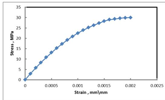
Fig. 3 Stress – Strain Curve for concrete
