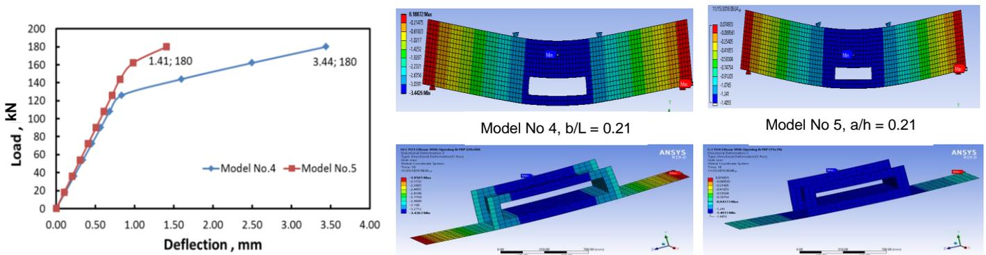
Fig. 14 Load deflections of RC beams with opening and CFRP and their patterns through numerical analysis
