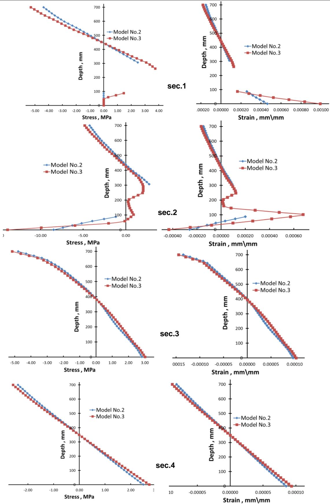
Fig. 12 Distribution of normal stress and normal strain for the selected sections in drilled RC beam
