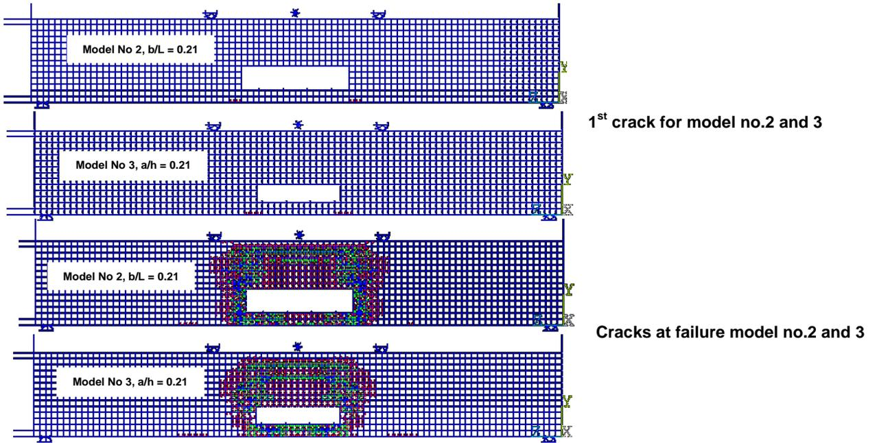
Fig. 13 Patterns of 1<sup>st</sup> crack and the cracks at failure for drilled RC beam, model No.2 and 3
