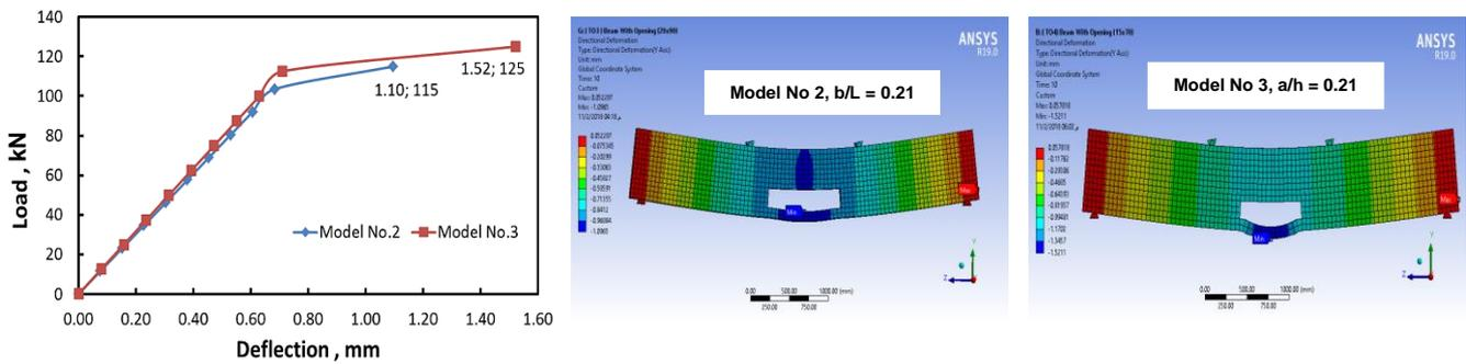
Fig. 11 Load - deflection of RC beams with opening and their patterns in numerical analysis
