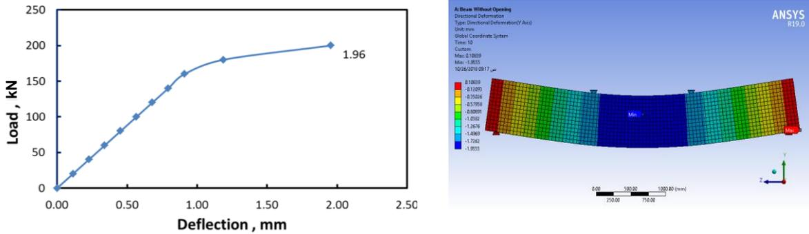
Fig. 7 Load - deflection of control RC beam and its pattern in numerical analysis
