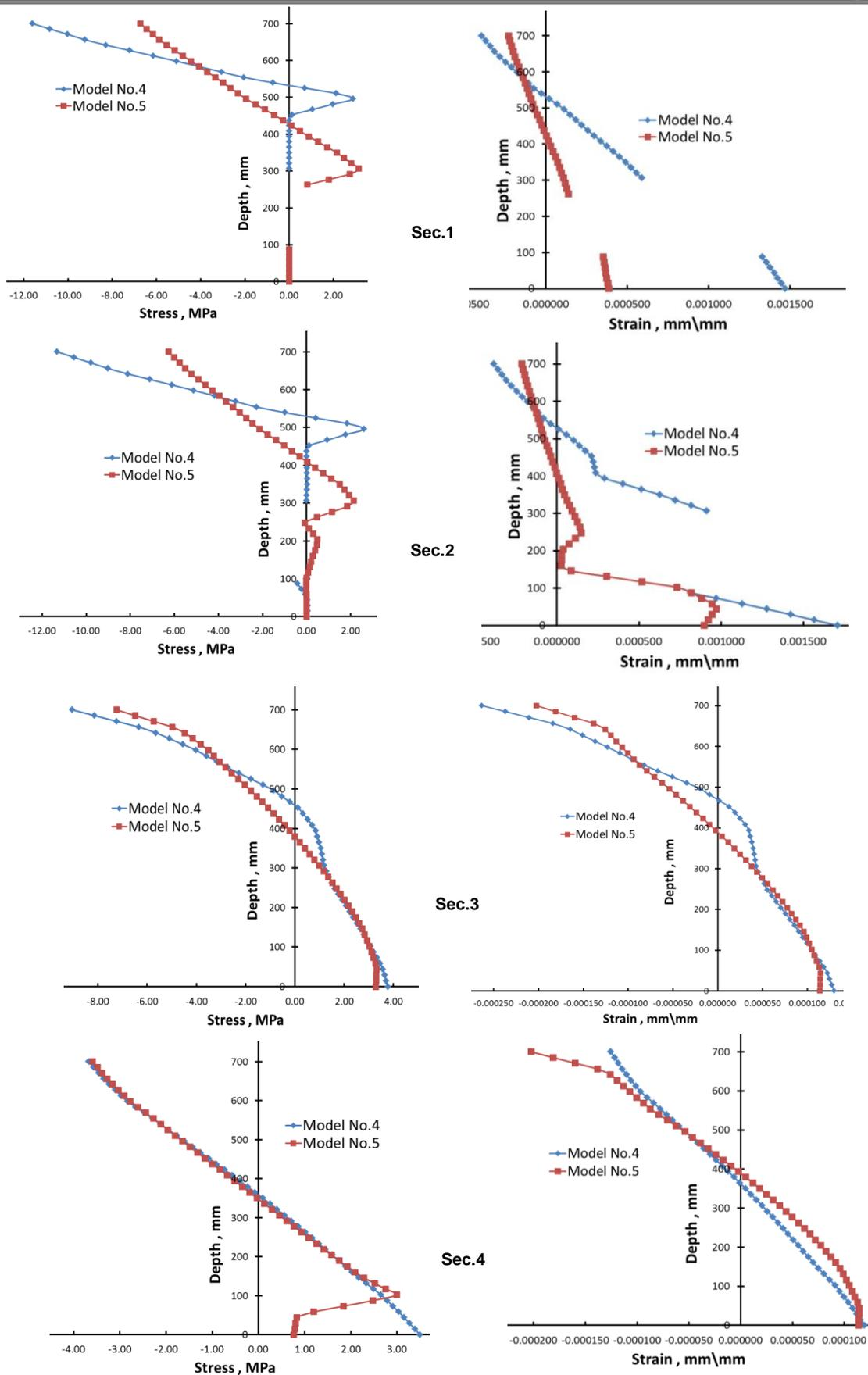
Fig. 15 Distribution of normal stress and normal strain for the selected sections in drilled RC beam
