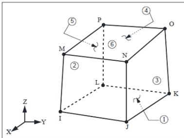
Fig. 1 SOLID65 concrete element
