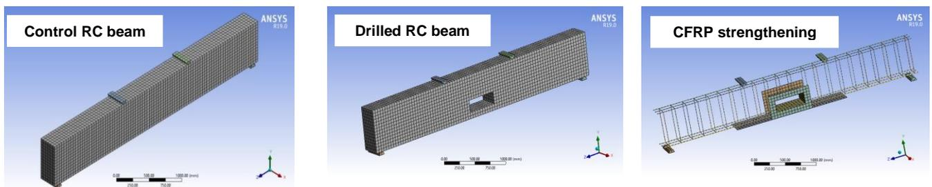
Fig. 6 Generated mesh for control RC beam, RC beam with opening and CFRP strengthening
