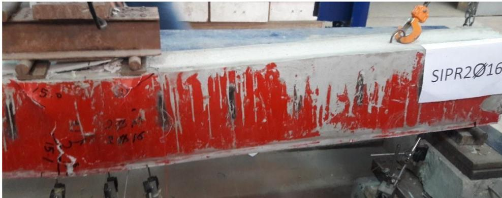
Fig.17: Failure mode of the specimens with FRP SIP forms, the second mode.
