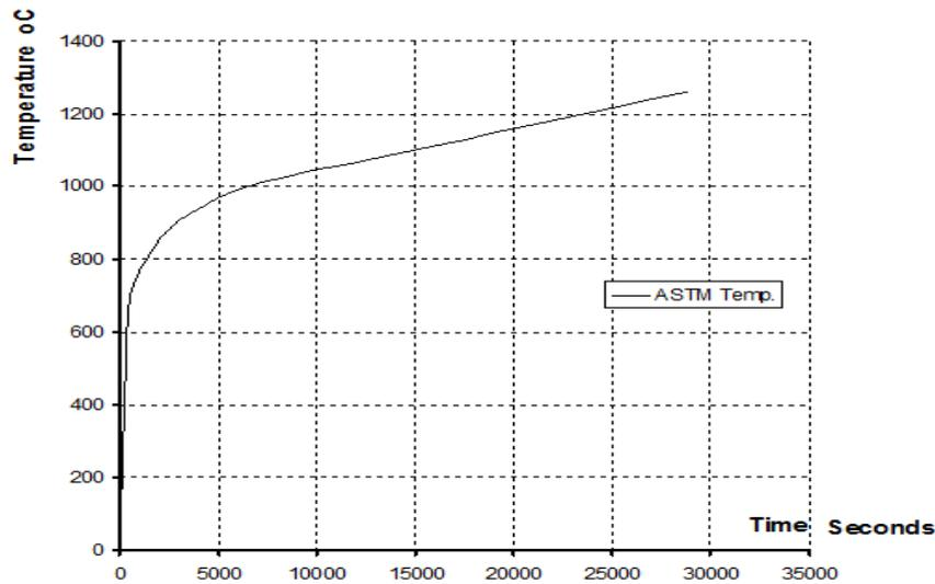
Fig. 2: ASTM 119 fire exposure testing curve[13]
