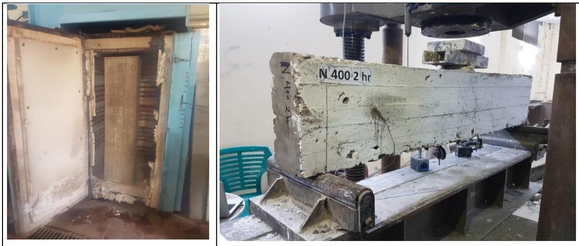
Fig. 3: Furnace and loading test setup.
