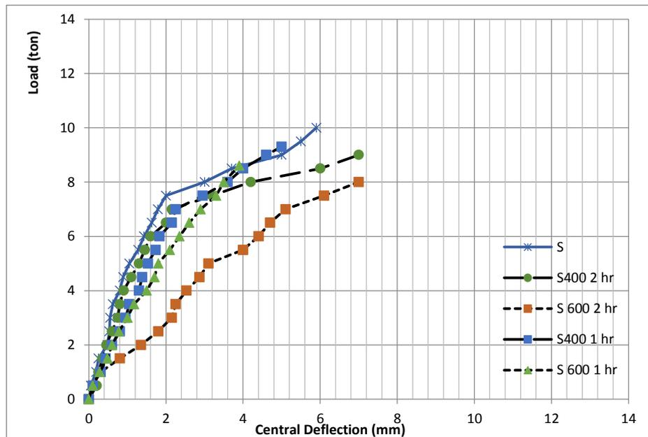
Fig. 8: Load deflection curve for self-compacting concrete beams under different level of temperature and different exposure time
