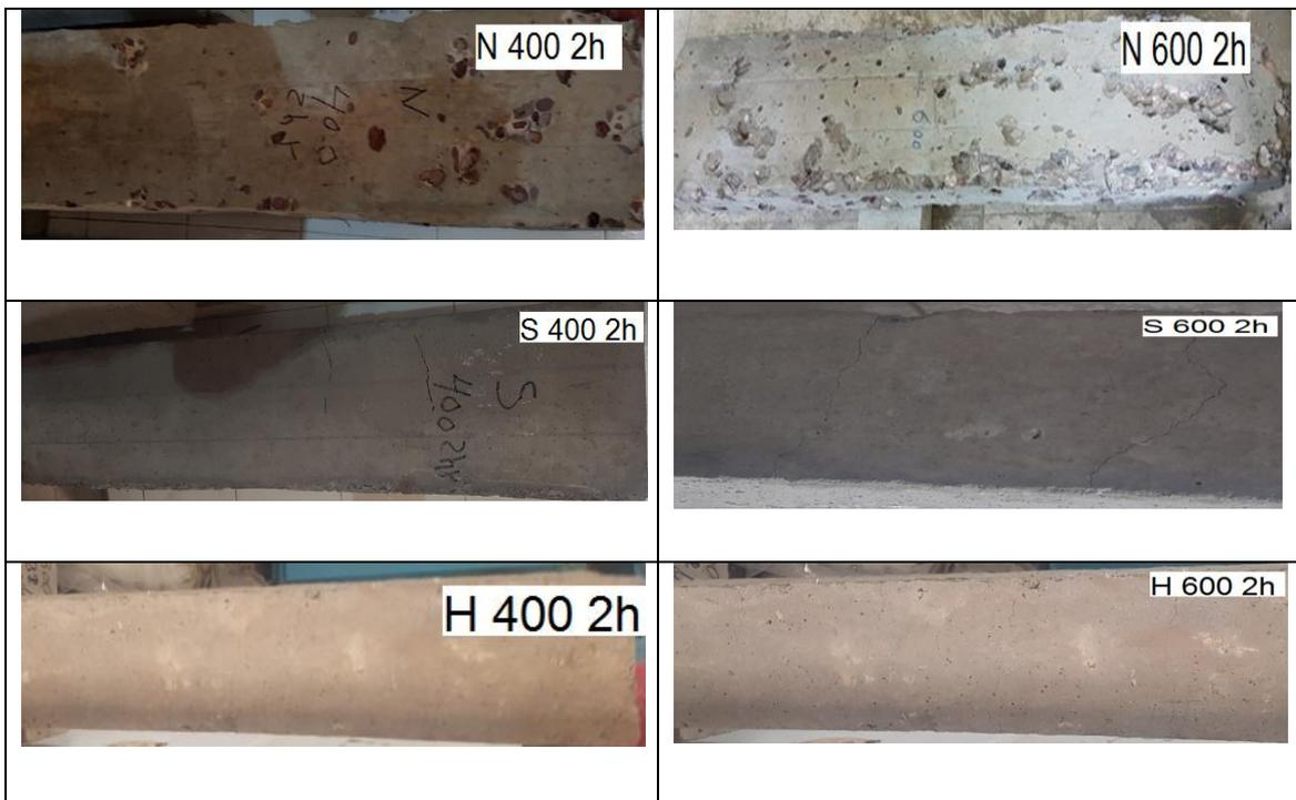
Fig. 5: Cracking phases for beams under different temperature for 2 hours exposure time
