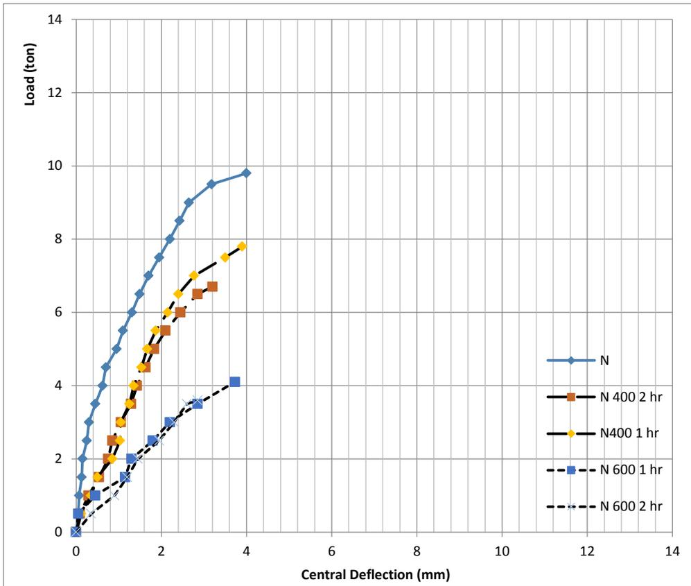
Fig. 7: Load deflection curve for normal concrete beams under different level of temperature and different exposure time
