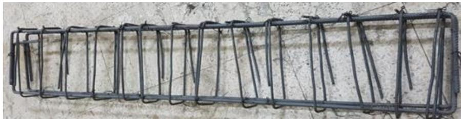
Fig. 1: Geometry and steel reinforcement for tested beam
