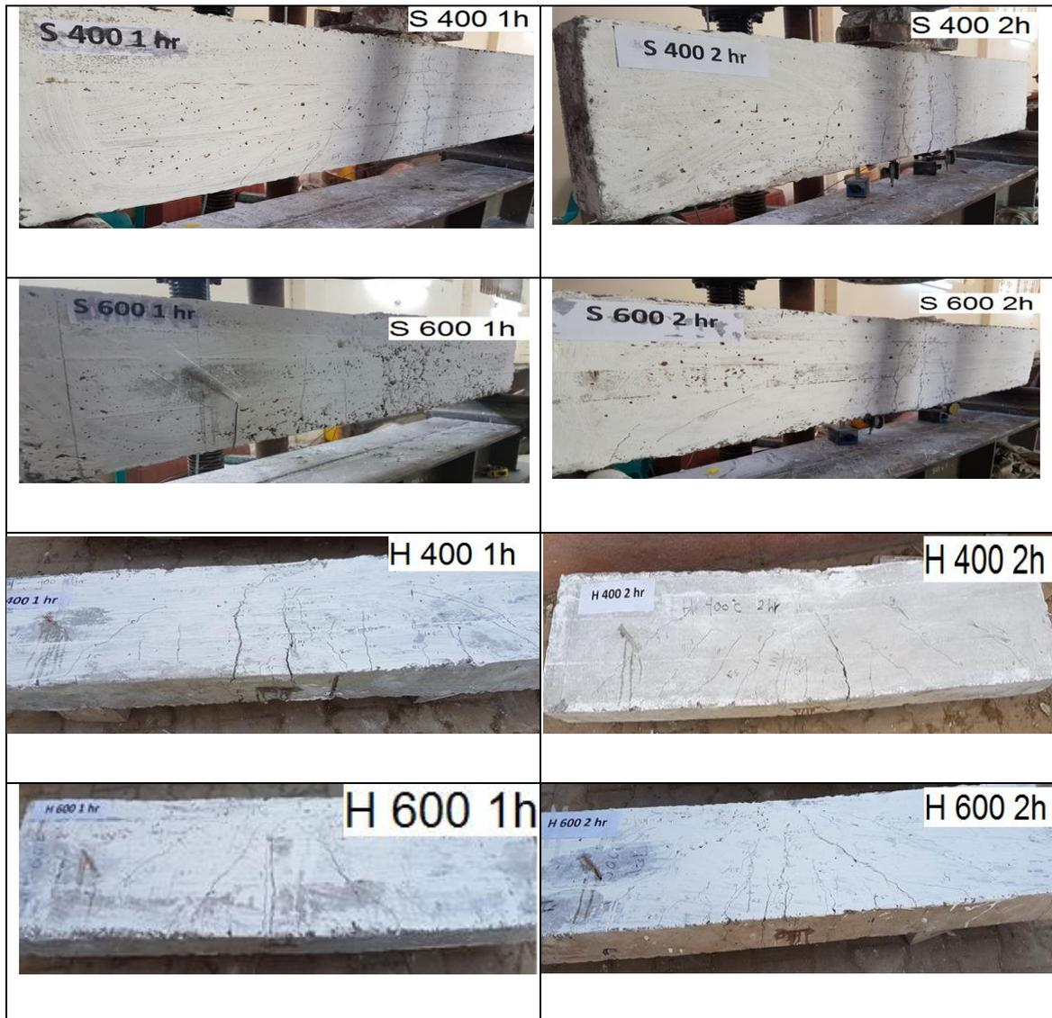
**Fig. 6: Crack pattern and mode of failure at different exposure time for NC, SCC and HSC beams**
