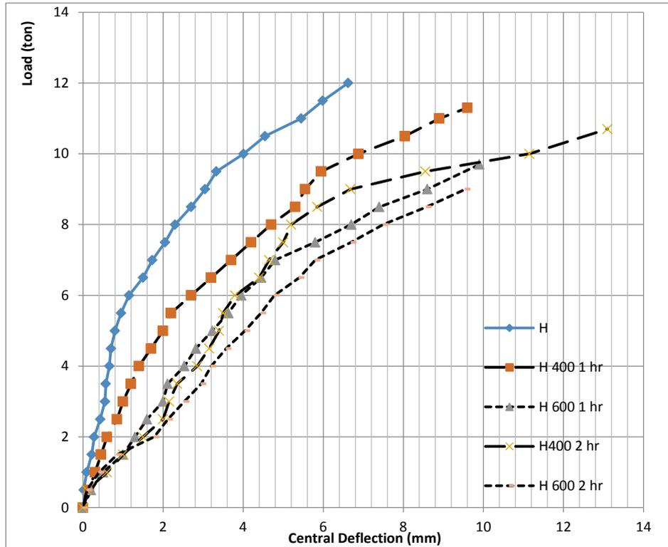
**Fig. 9: Load deflection curve for high strength concrete beams under different level of temperature and different exposure time**
