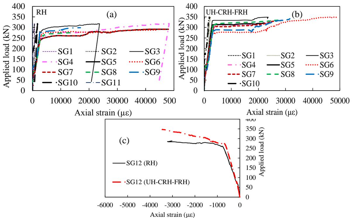
Fig. 4: Applied load versus the tensile axial strain (a) RH beam, (b) the semi-precast beam, and (c) the compression strains for the RH and UH-CRH-FRH beams
