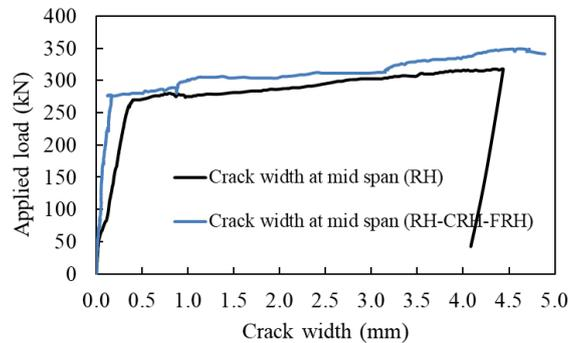
**Fig. 5: Applied load versus crack width at the beam mid span**
