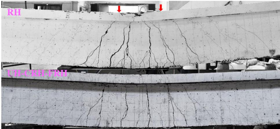
Fig. 3: Final failure mode of the test beams
