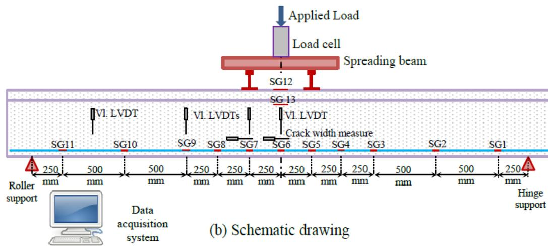
Note: VI. LVDT is vertical linear variable displacement transducer and SG is strain gauge
