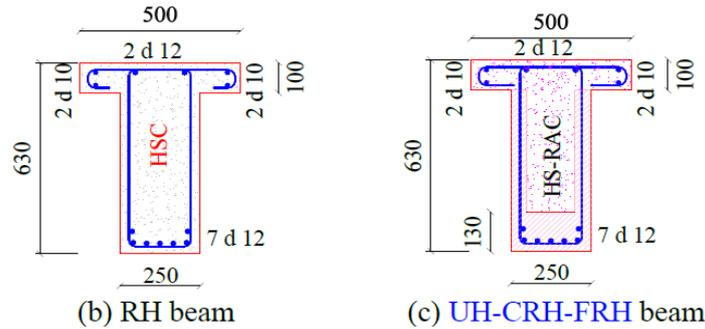
Fig. 1: Schematic drawings for the reinforcement details and concrete dimensions
