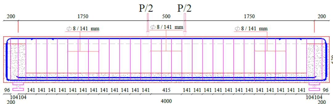
(a) Reinforcement details of all beams
