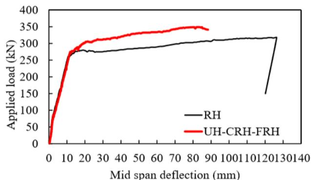
**Fig. 6: Load versus deflection at the beam mid-span**
