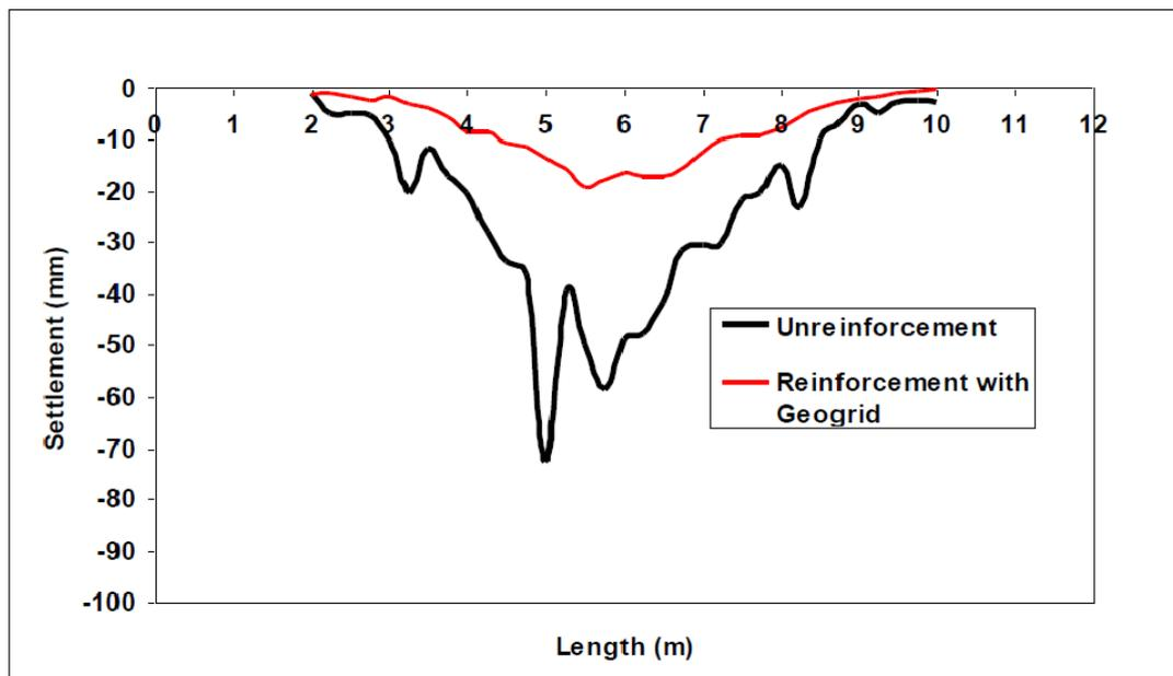
**Fig.7: Monitoring Displacements at Surface after Reinforcement with One Layer of Geogrid**
