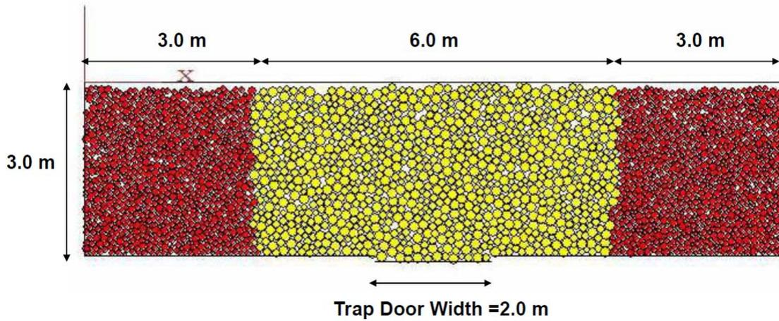
Fig.1: Trap Door Model Using PFC2D
