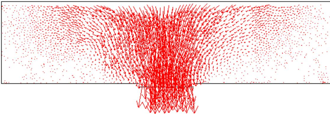
**Fig.6: Displacement Vectors After Trap Door Movement**
