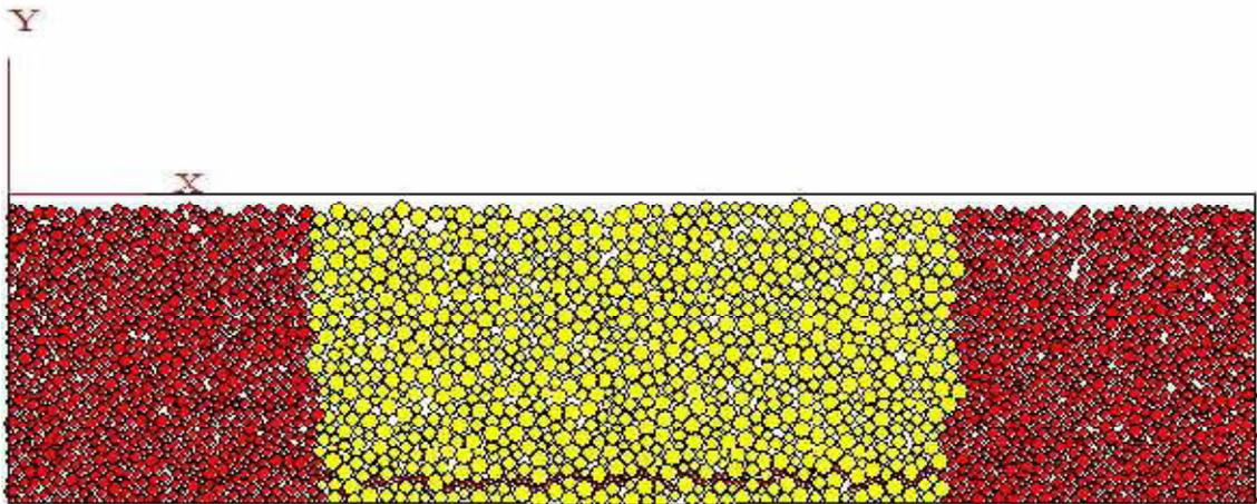
**Fig.3: Model with One Layer of Geogrid**
