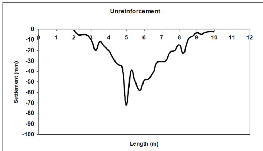
Fig.5: Monitoring Displacements at Surface after Trap Door Movement
