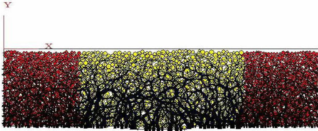
Fig.4: Contact Force After Cycling the Model under Gravity
