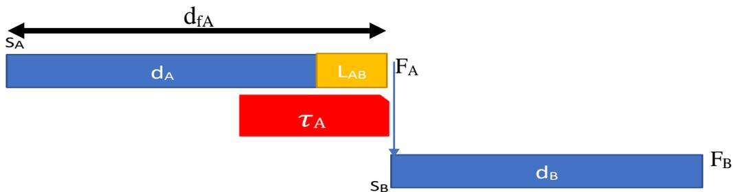
Fig. 4. The Precedence Constraint for the FS Relationship
