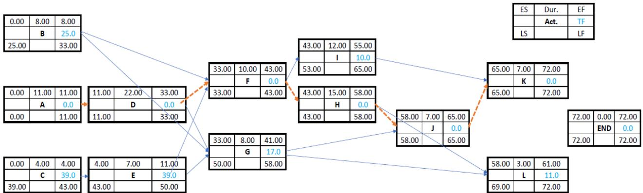
Fig. 2. Probabilistic Network Diagram
