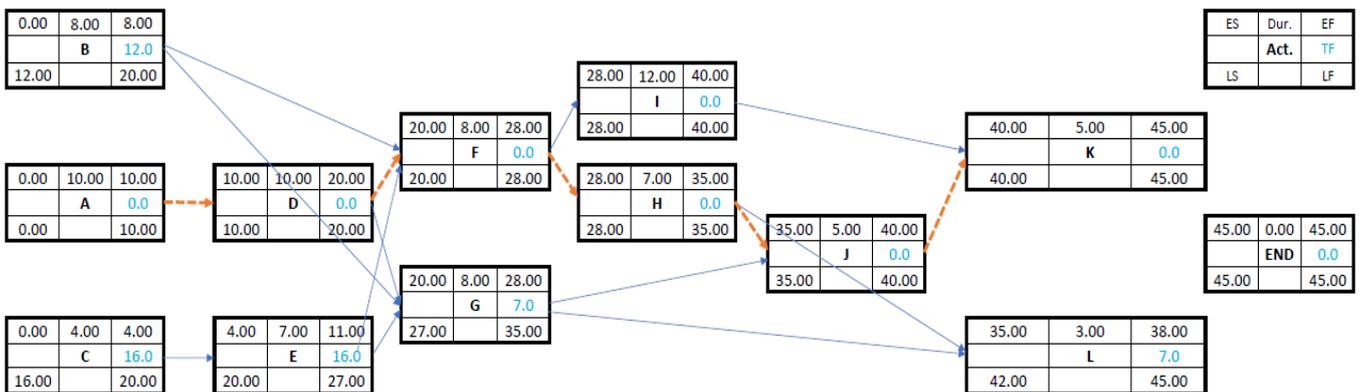
Fig. 6. Probabilistic Crashed Network Diagram without Float Consumption
