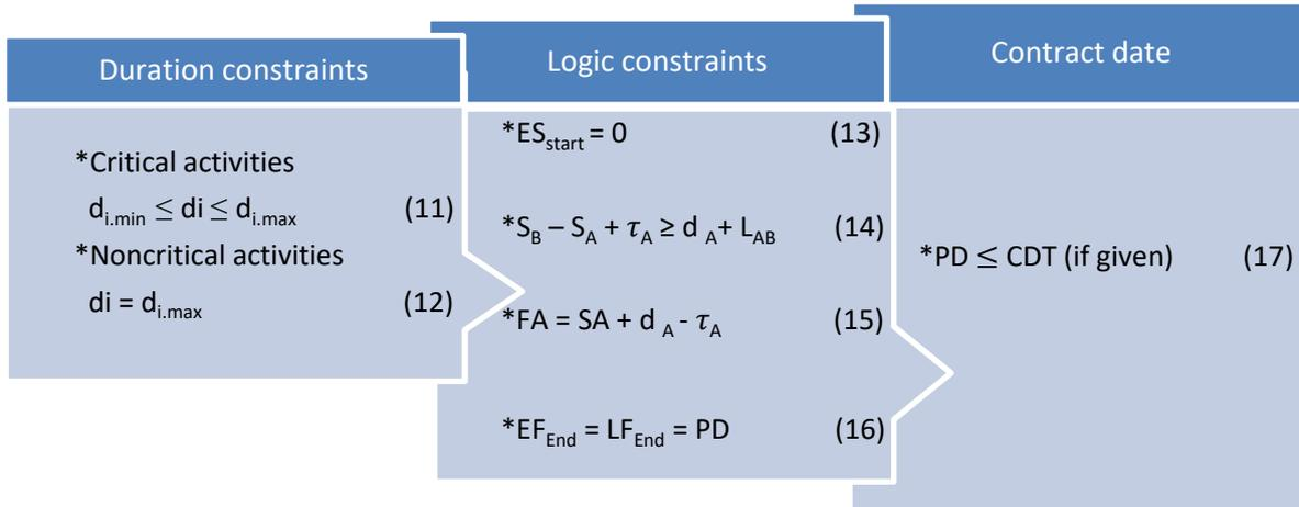
Fig. 3. Types of the Model Constraints
