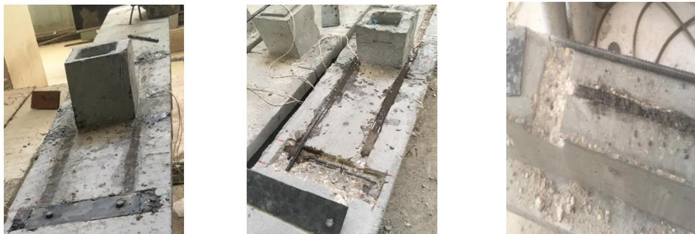
Fig. 2. Shape of the grooves and steel anchors for the strengthened beams with NSM bars.
