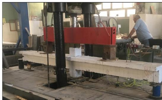
**Fig. 3.** System of loading on beams.
