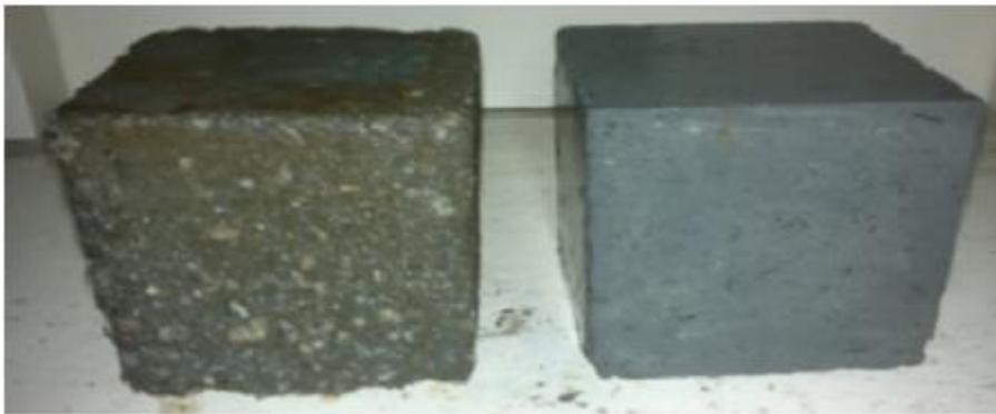
Fig. 6. Visual appearance of BFAGC and OPC concrete after 18 months [71].
