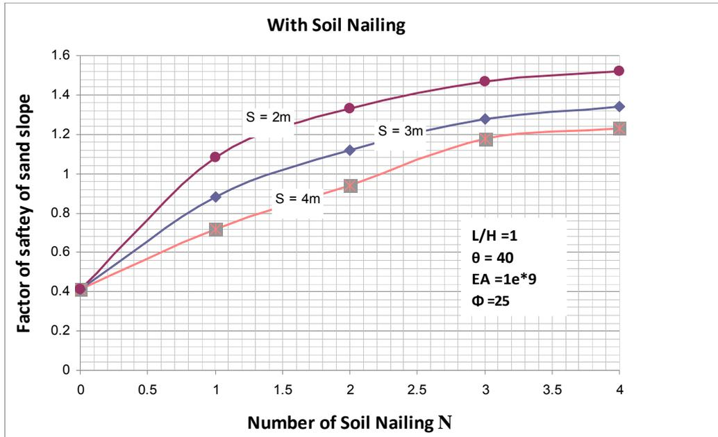
Fig. 9 Factor of safety of sand slope under earthquake loading with soil nailing versus different number of soil nailing and the horizontal spacing in the long direction
