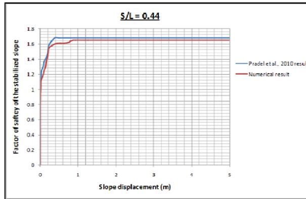
Fig. 4 Comparison of 3D FLAC program results with the 2D PLAXIS modeling results for S/L =0.44, (After Pradel et al., 2010)
