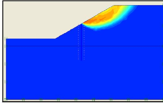
Fig. 3 The shape of the slip surface of the stabilized slope using the numerical 2D PLAXIS modeling
