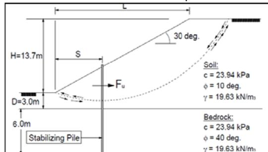
Fig. 1 Stabilized slope geometry and its material properties (After Pradel et al., 2010)
