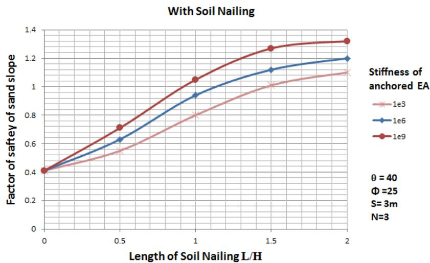
Fig. 9 Factor of safety of sand slope under earthquake loading with soil nailing versus different length of soil nailing and the stiffness of anchored
