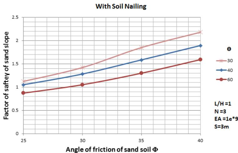
Fig. 8 Factor of safety of sand slope under earthquake loading with soil nailing versus different angle of friction and the slope angle
