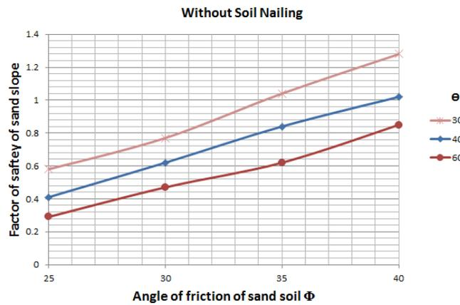
Fig. 7 Factor of safety of sand slope under earthquake loading without soil nailing versus different angle of friction and the slope angle
