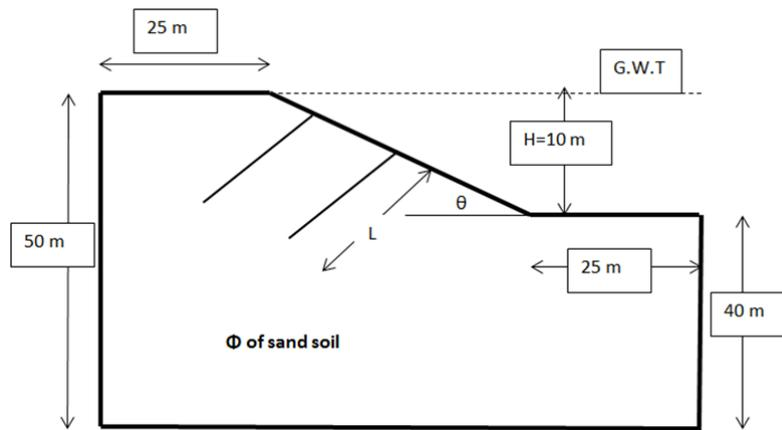
Fig. 5 The geometry model for different studied parameters in 2D PLAXIS model
