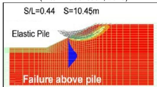
Fig. 2 The shape of the slip surface of the stabilized slope using the 3D FLAC program (After Pradel et al., 2010)
