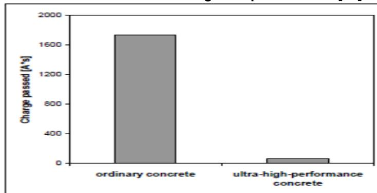
Fig.8. Rapid, the 'diffusion' front of chloride ions was visualized using a special staining method chloride permeability test [66] results for the internal UHPC mixture M1Q and normal concrete acc. EN 206.
