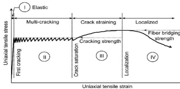
Fig. 17 Idealized uniaxial tensile response of UHPC [115].
