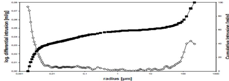
Fig.7. Mass Pore-size distribution of the internal UHPC mixture M1Q. The low total porosity and particularly the very low amount of capillary pores are the reasons for UHPC's enhanced long-term performance [66].
