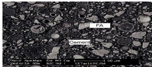
Fig. 18 Microstructure of UHPC paste containing FA and SF, w/b=0.18, 28d [19]
