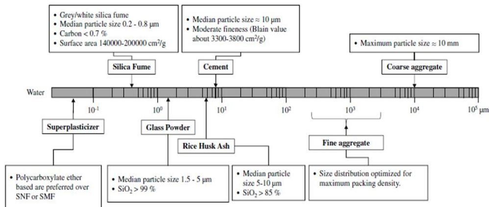
**Fig. 9. Size distribution of constituents of UHPC [adapted from Materials and Structures[1,28]**
