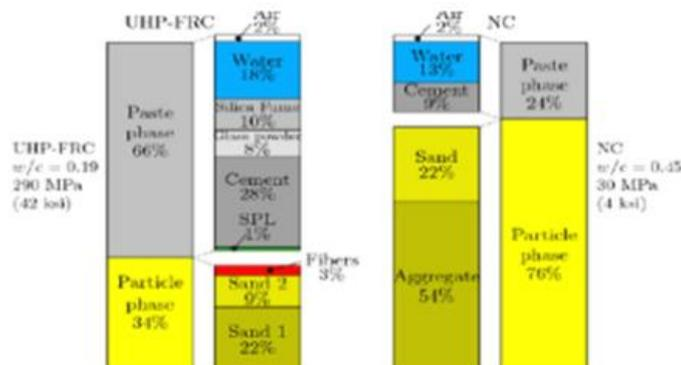
Fig. 5. Example of mix proportions by volume comparing UHPFRC with normal concrete [29]
