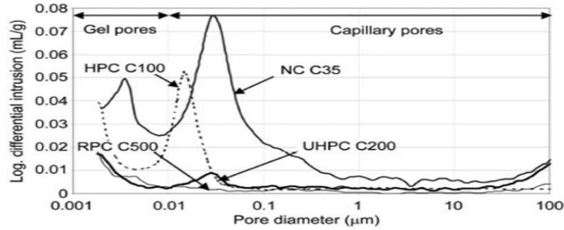
Fig.13. Pore size distribution of UHPC, HPC and NC [110].
