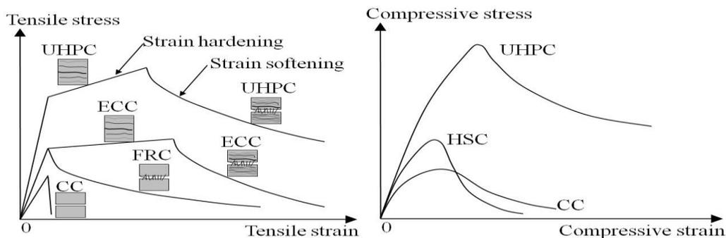
**Fig.1 Typical response of UHPC in uniaxial stress state compare with conventional concrete (CC), high-performance concrete (HPC), fiber-reinforced concrete (FRC), and engineered cementitious composites (ECC): (a) uniaxial tension, (b) uniaxial compression [16].**
