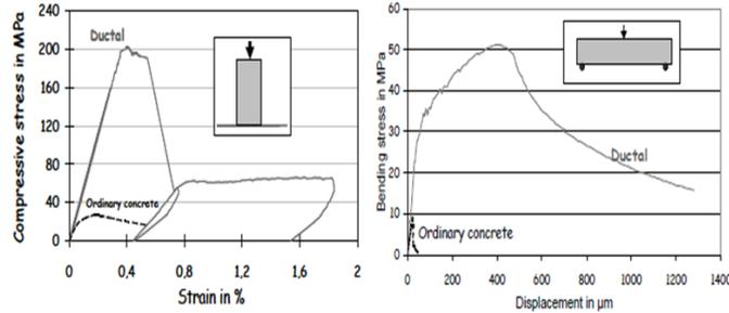
Fig. 4. Figure 11 Ductal® behaviour in compression (left) and in bending (right) [37]
