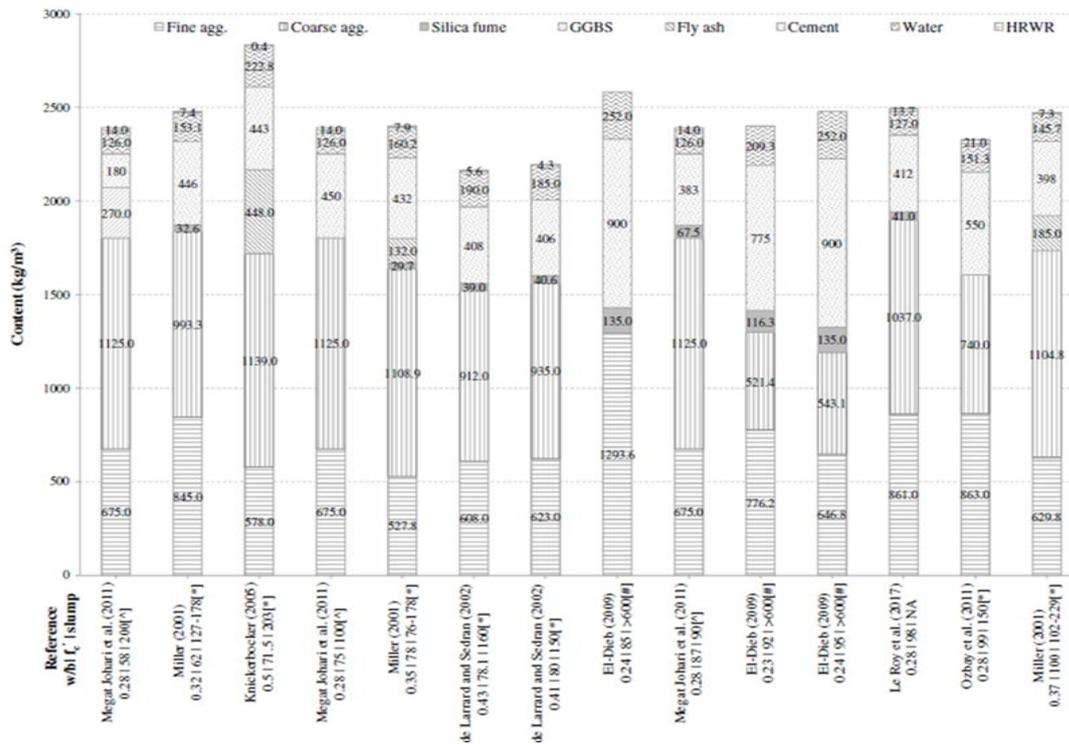
Fig. 10 Materials and mixture proportions of UHPC: reference, w/c, compressive strength (f'c), and slump presented below each mixture; % fiber content shown in box on top [1].
