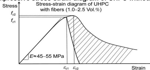
**Fig.16 Compressive stress-strain-diagram of UHPC with fibers [112]**
