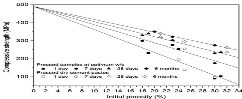
**Fig.12. Strength-porosity relationship of pressed and dry cement pastes at different ages (data from Bajza 1972) [98].**
