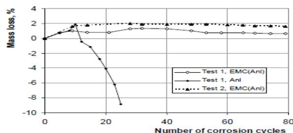
Fig. 6. Mass loss of the concrete versus number of corrosion cycles [59]
