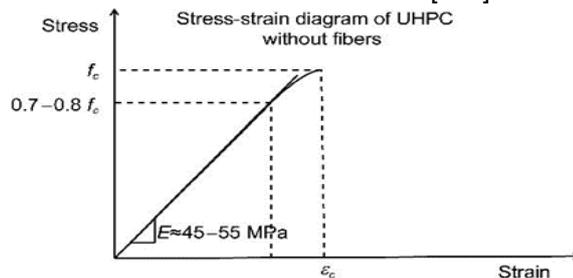
**Fig. 15 Compressive stress-strain-diagram of UHPC without fibers [112]**
