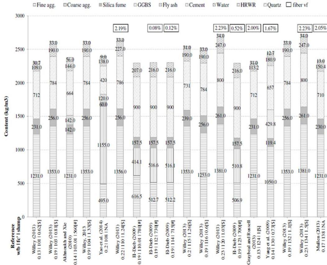
**Fig. 11. Materials and mixture proportions of UHPC: reference, w/c, compressive strength (f'c), and slump presented below each mixture; % fiber content shown in box on top [1]**
