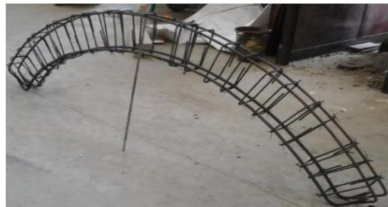
**Fig. 4(c) Reinforcing steel cage of BCP-D10-R60.**
