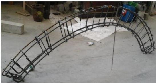
**Fig. 4(b) Reinforcing steel cage of BCP-D15-R60.**
