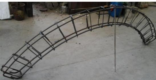
**Fig. 4(d) Reinforcing steel cage of BCS-C-R60.**
