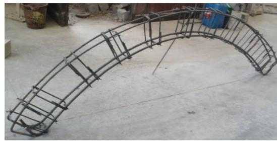
**Fig. 4(e) Reinforcing steel cage of BCP-D20-R60.**
