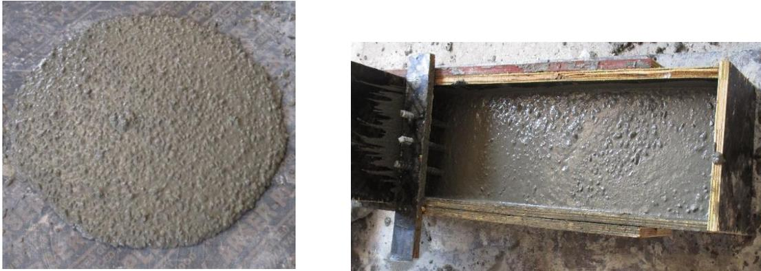
**Fig. 5** Flow ability of the used self-compacted concrete.
