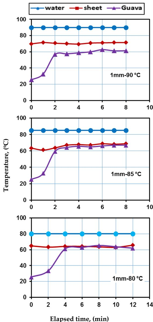
Fig. 5. Water, Sheet and Guava puree temperatures as affected by elapsed time at 1mm thickness.
