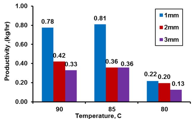
Fig. 9. Productivity (kg/h) of Guava dried as affected by water basin temperatures and puree thickness for all drying experiments.
