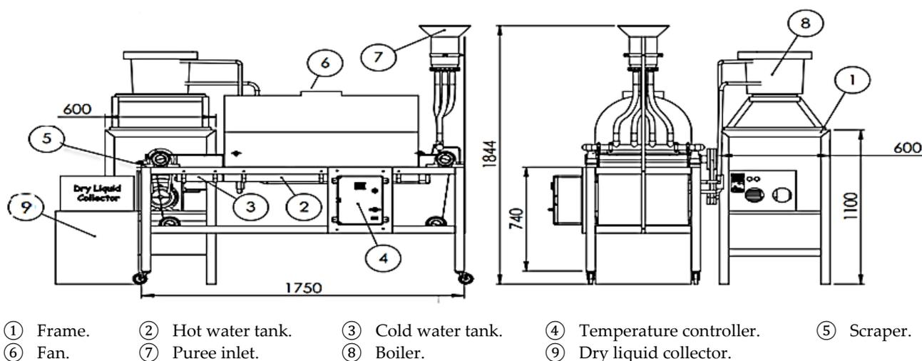
Fig. 1. Elevation and side view of (RW) dryer structure.
