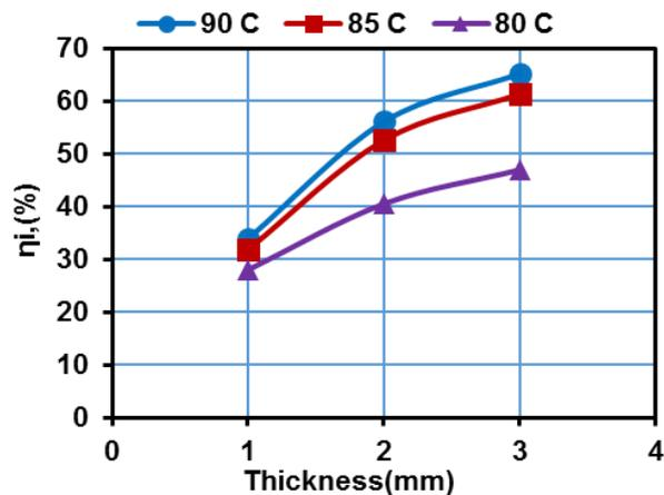
Fig. 8. Drying efficiencies of Guava puree as affected by puree thickness, water basin temperatures.
