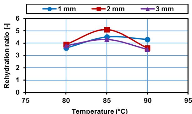
Fig. 11. Rehydration ratio for drying Guava at all drying conditions studied.
