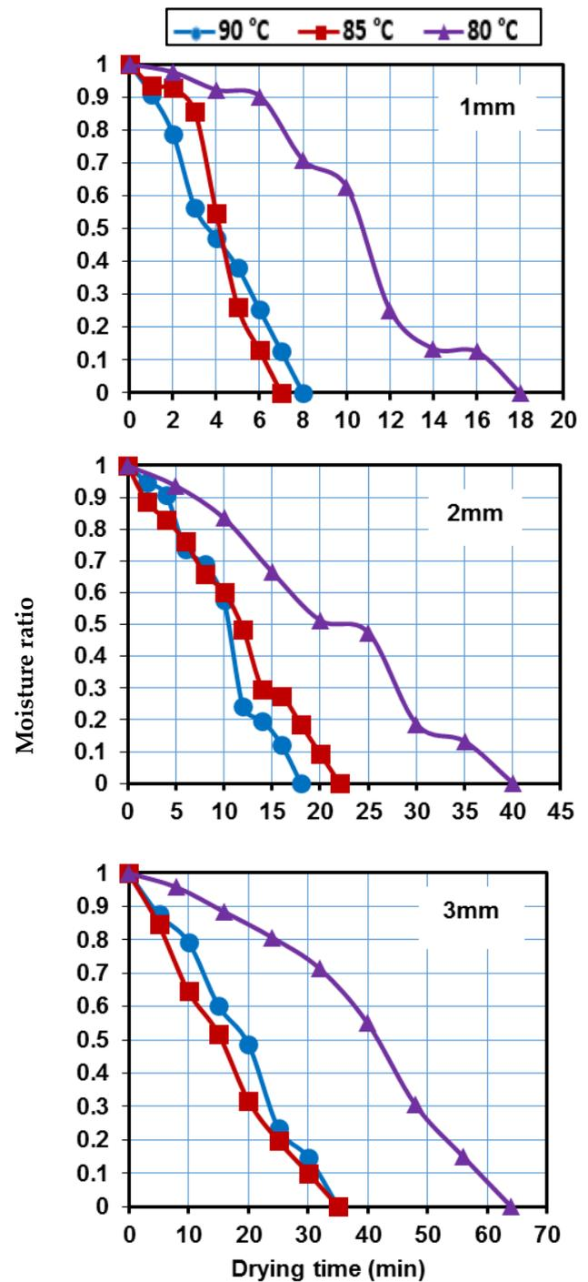
**Fig. 3.** Moisture ratio of Guava puree as affected by water basin temperature and drying elapsed time at the three different thicknesses studied.
