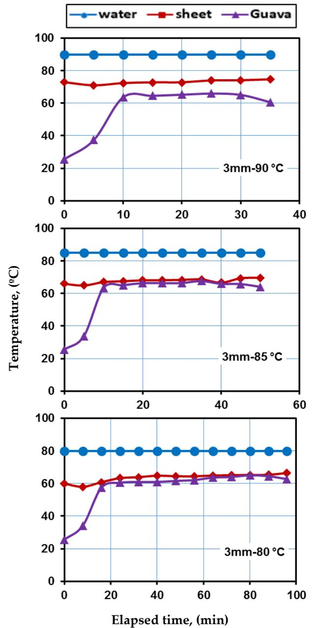
Fig. 7. Water, Sheet and Guava puree temperatures as affected by elapsed time at 3mm thickness.
