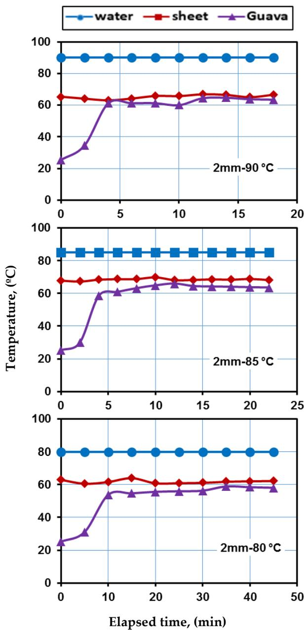
Fig. 6. Water, Sheet and Guava puree temperatures as affected by elapsed time at 2mm thickness.
