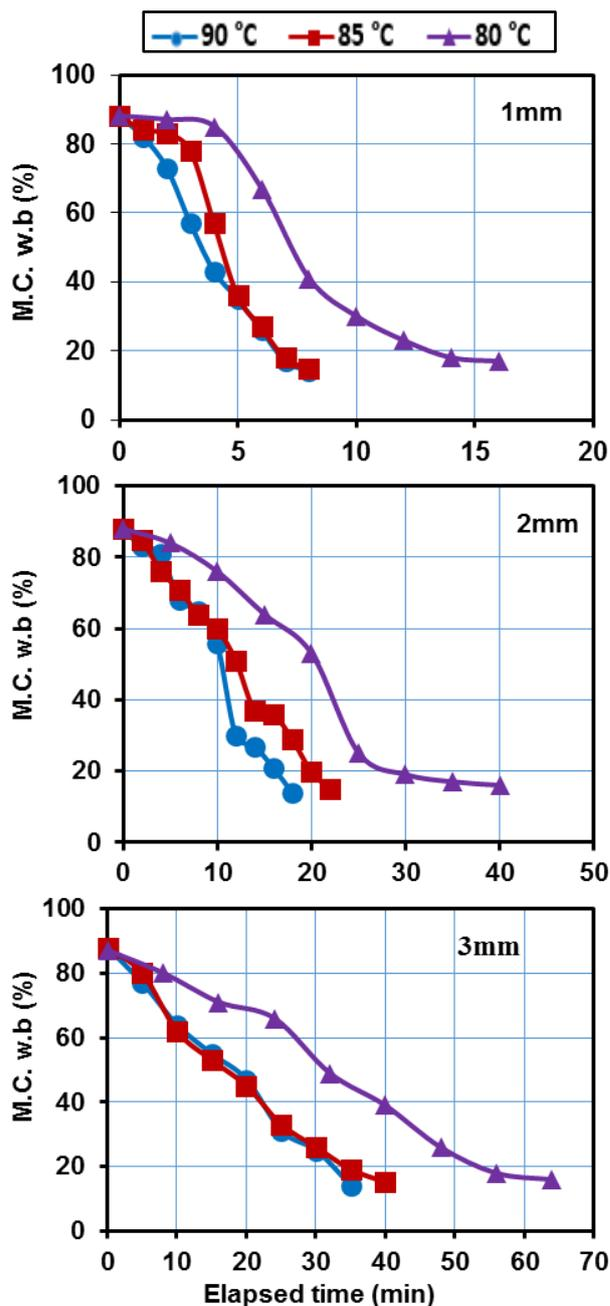
Fig. 2. Moisture contents wet basis (%) of Guava puree as affected by water basin temperature and drying elapsed time at the three different thicknesses studied.
