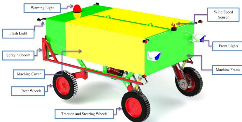
Figure 7. The main components of the spraying robot.
