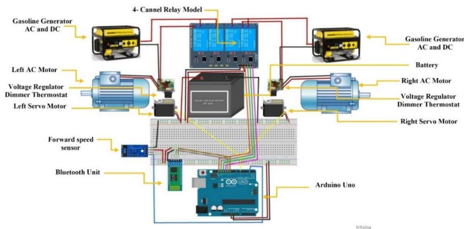
Figure 1. Electronic circuit components.
