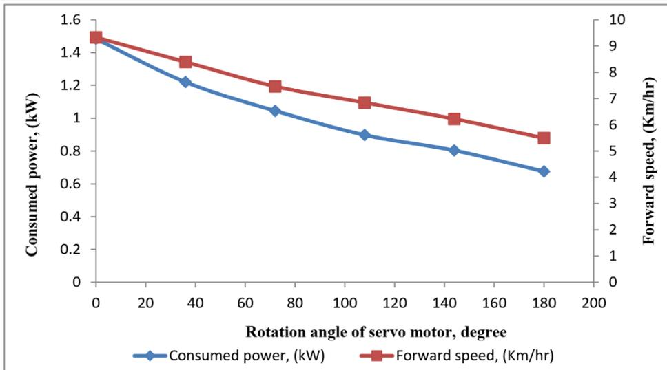
Figure 9. The relation between the forward speed, power consumed, and the servo motor rotation angle for one generator.
