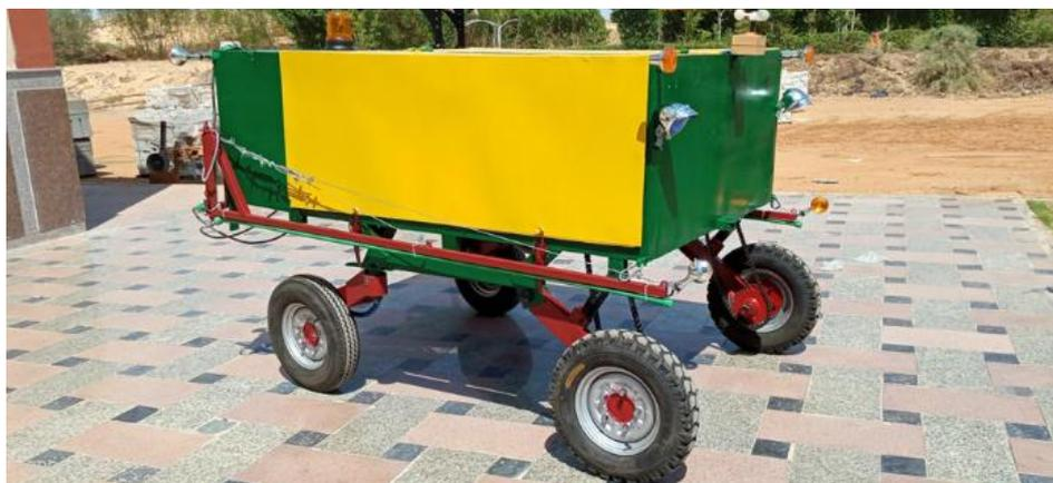
Figure 4. The spraying robot with a non-spraying position.
