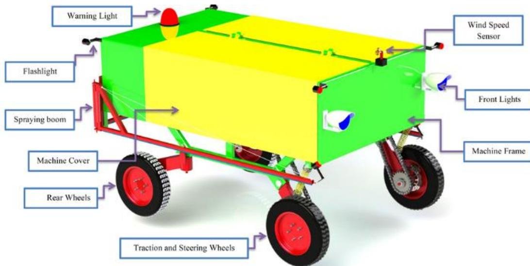
Figure 3. The isometric view of the spraying robot shows the main components with a non-spraying position.
