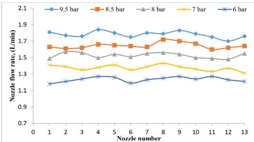
Figure 9. Distribution Uniformity of spraying machine for nozzle type (422HCC03).
