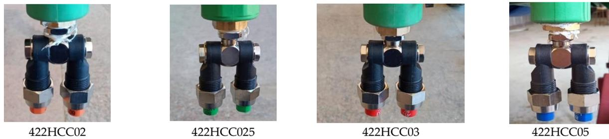
Figure 2. The different types of hollow cone ceramic nozzles are used in the current study.
