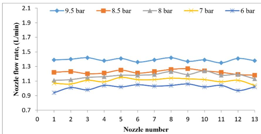
**Figure 7.** Distribution Uniformity of spraying machine for nozzle type (422HCC02).
