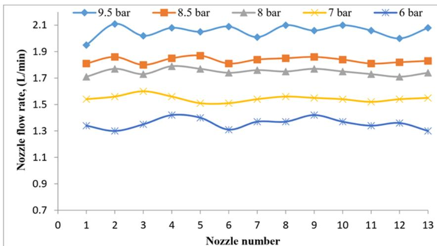
Figure 10. Distribution Uniformity of spraying machine for nozzle type (422HCC05).
