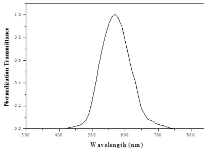
**Fig. 4.** Optical transmission spectra of  $2.5\text{Cu}_2\text{O}$ .
