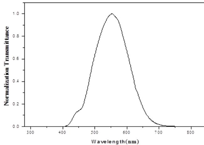
**Fig. 3.** Optical transmission spectra of collected sample ( $1\text{Cu}_2\text{O} + 1.5 \text{Fe}_2\text{O}_3$ ).
