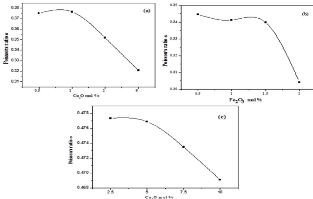
Fig. 9 (a-c) the variation of Poisson's ratio with composition a) with Cu<sub>2</sub>O mol% b) with Fe<sub>2</sub>O<sub>3</sub> mol% c) with Cu<sub>2</sub>O mol%.
