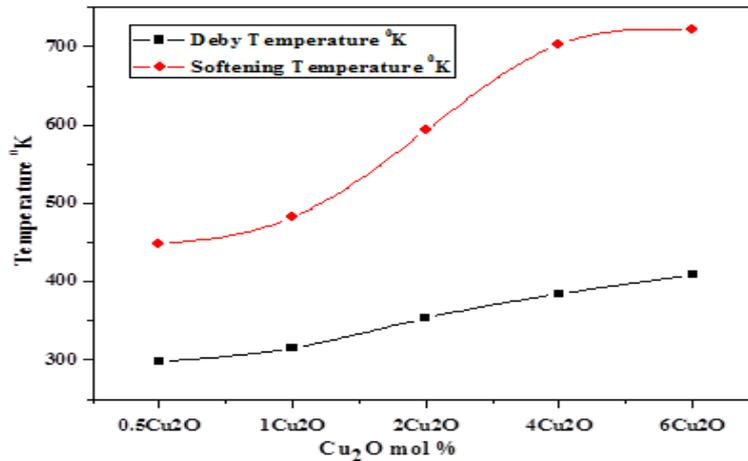
Fig. 8. The relation between Debye temperature, Softening temperature and Cu<sub>2</sub>O content.
