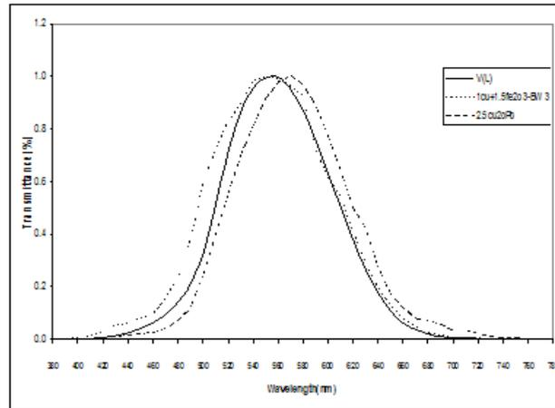
**Fig. 5.** Shows Normalized spectral responsivities graph as a function of wavelength for 2 composition 1Cu+1.5Fe<sub>2</sub>O<sub>3</sub>& 2.5Cu<sub>2</sub>OPb (at band width 1nm) compared with CIE V (λ) filter.
