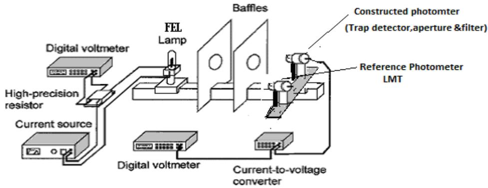
Fig. 1. Schematic diagram for the Photometric Measurement System.
