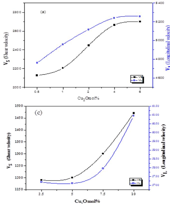
**Fig. 6. (a-c):** Variation of the longitudinal  $V_L$  and shear velocity  $V_S$  a) with  $\text{Cu}_2\text{O}$  mol % b) with  $\text{Fe}_2\text{O}_3$  mol % c) with  $\text{Cu}_2\text{O}$  mol %.
