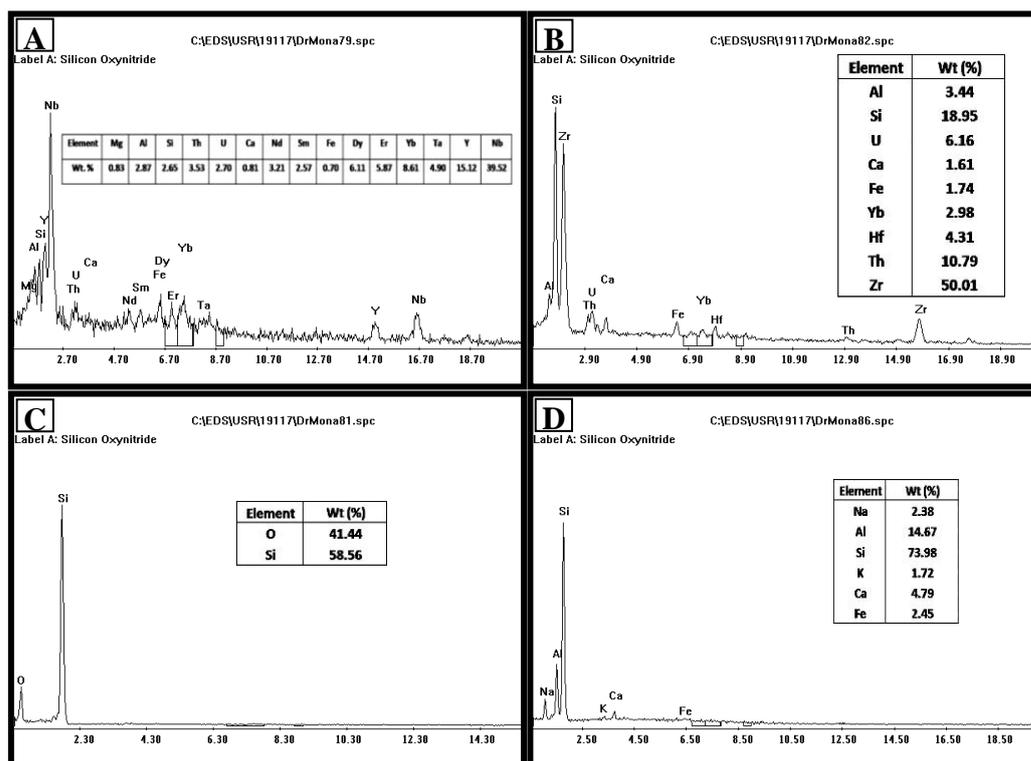
Fig. 1: EDX analysis data of fergusonite A, zircon B, quartz C, and feldspar D.
