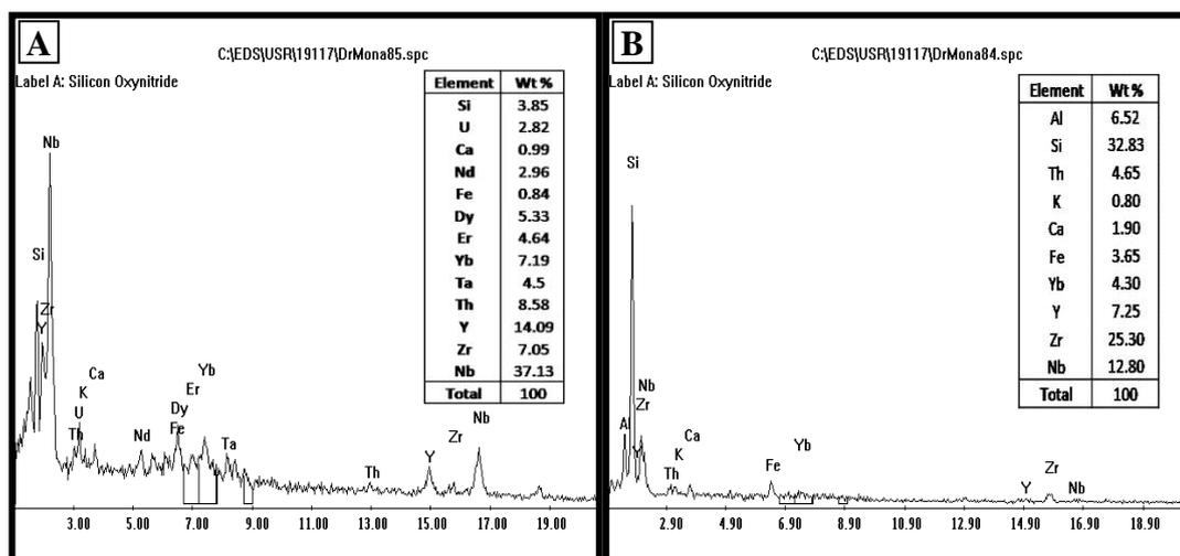
Fig. 10: EDX analysis data of froth (A), sink (B) products.
