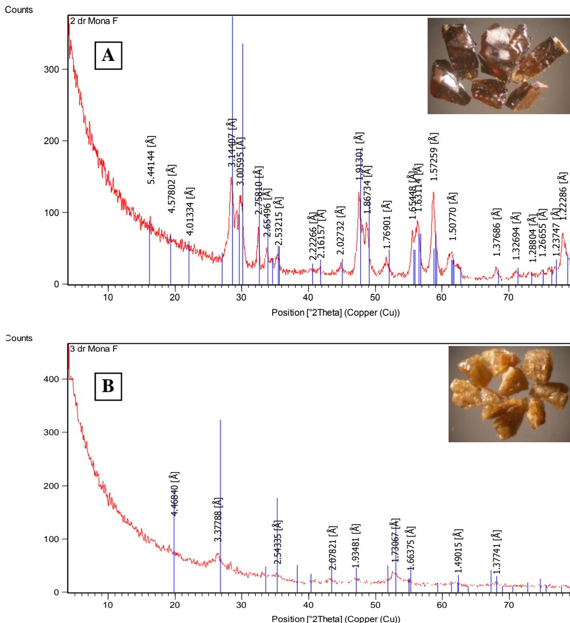
**Fig. 2: X-ray diffraction patterns; (A) fergusonite (ASTM card no. 9-0443), (B) zircon (ASTM card no.01-081-0591).**
