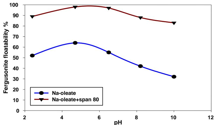
Fig. 5: Effect of pH on floatability of fergusonite surface using Na-oleate and the mixture collectors.
