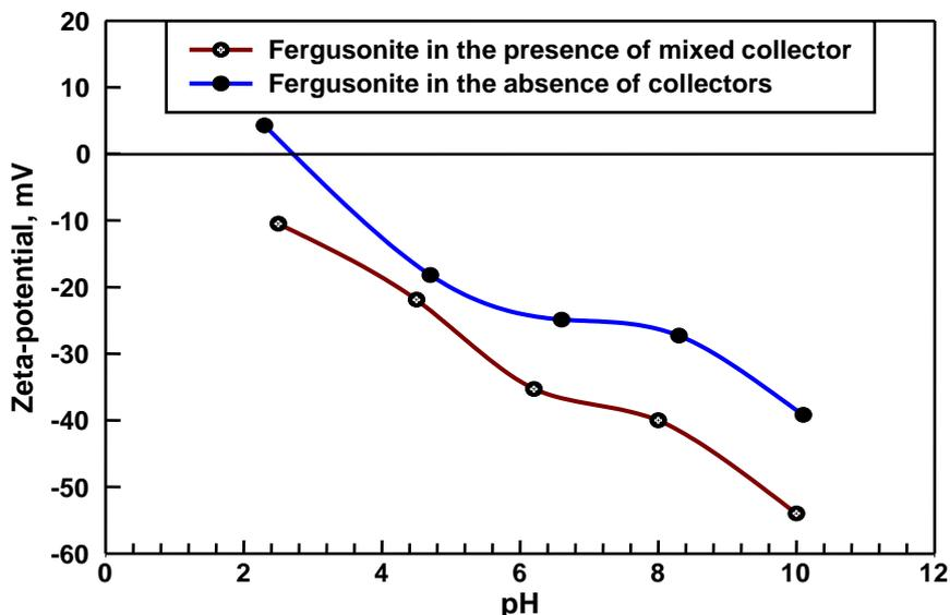
Fig. 7: Effect of mixture of sodium oleate and span 80 on zeta-potential of fergusonite.
