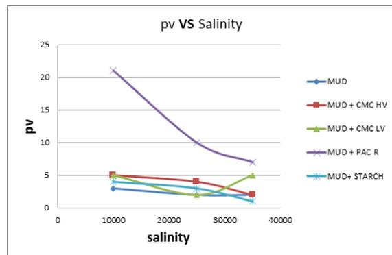
**Fig. 2:** Salinity concentration vs. PV for four types of polymers.
