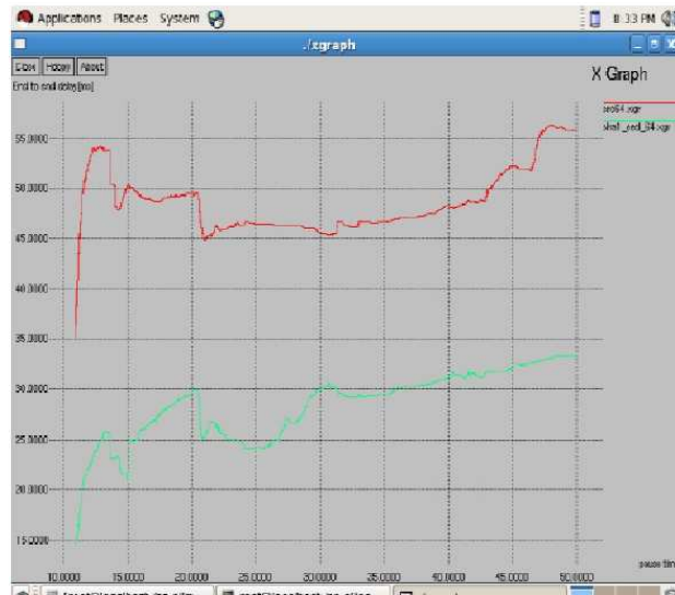
Fig. 4: End to End delay of CRC-32 and SHA-1 at 64 bit key
