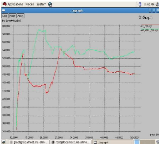
Fig. 6: End to End Delay of CRC-32 and SHA-1 at 256 bit key
