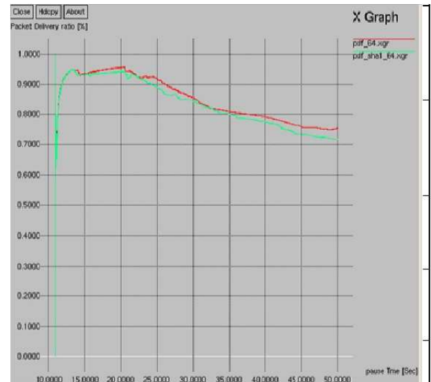
Fig. 8: Packet delivery ratio of CRC-32 and SHA-1 at 64 bit key
