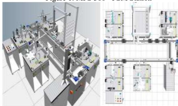
Finally, the sorting station will have the task of sorting the jacks according to their nature (the red plastic station, black plastic or metallic coating).
