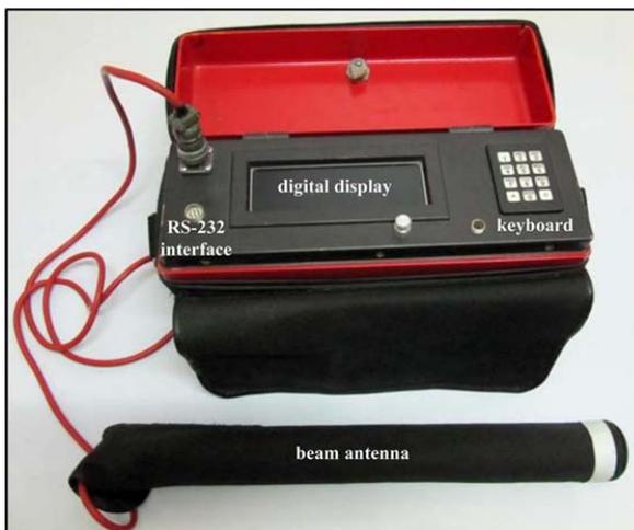
Fig. 2: The Cerescope device used in the present study
