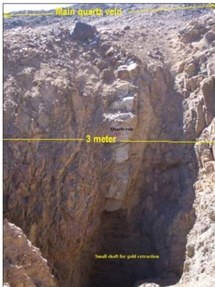
Fig. 8: Small shaft in the first zone of old working to follow the quartz vein for gold exploitation. After Ahmed (2012).
