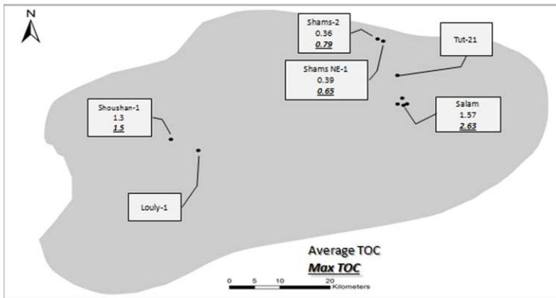
Fig. 6: TOC limits (wt %) for Abu Roash Formation in Shoushan Basin.
