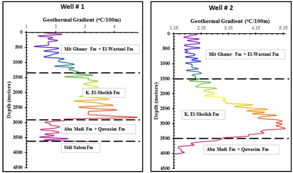
Fig.12: Well#1 and Well#2 geothermal-lithological zonation.
