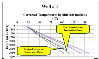
Fig. 5: Plot showing the Uncorrected and Corrected Temperature Curves versus depth.
