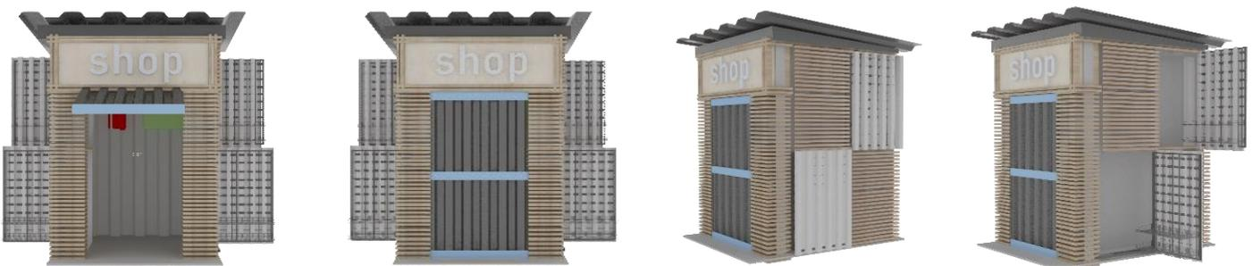
Figure 11: A model of the proposed commercial unit and the method of opening and closing it.
