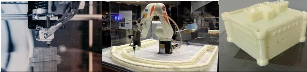
3D model of the castle using 3D printer
