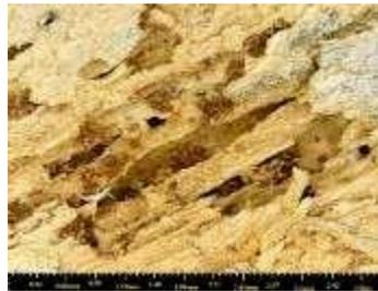
**Figure (3-4) digital microscope image** from Figure (3-1) shows that biological deterioration (holes, tunnels) and defiberation.
