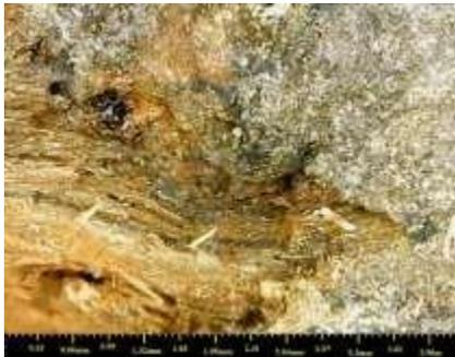
**Figure (2-4) digital microscope image** from Figure (2-2) shows that corrosion layer and accumulation of salts crystals inside the wood texture.
