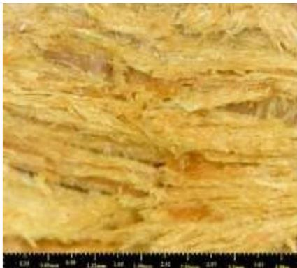
Figure (4-2) digital microscope Figure from figure (4-1) shows that breaking, secessions, castrate in the fiber as a result to temperature.
