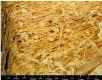
**Figure (1-4)** digital microscope detail of figure (1-1) shows defiberation and crystallization of salts on cellulose fibers.
