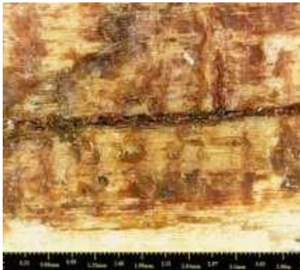
**Figure (5-4) digital microscope** Figure from Figure (5-2) shows that some cracks, corrosion and defiberation.
