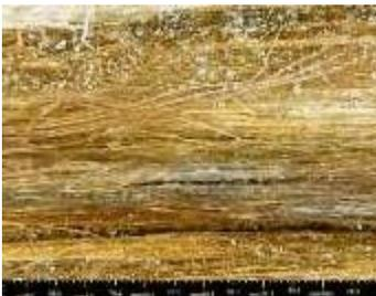
**Figure (1-5) digital microscope detail of figure(1-2) shows salt crystals found on the surface of wood and defibration resulting from the effect of salts.**
