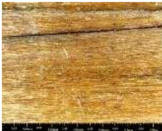
**Figure (3-5) from Figure digital microscope image (3-2)** shows that cracks there is biological deterioration (holes, tunnels and different colors).
