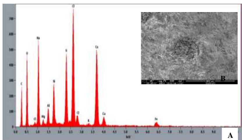
Fig.5 shows analysis and investigation of preparation layer in the mask A) EDS pattern B) SEM photomicrographs of preparation layer distribution on the surface.
