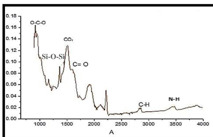
Fig. 8 shows the FTIR spectra of the black pigment of the mask and identification of binding media and layers of ground
