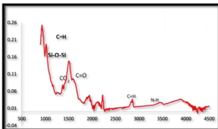
Fig.11 the FTIR spectra of the red pigment of the mask, identification of binding media, and layers of ground
