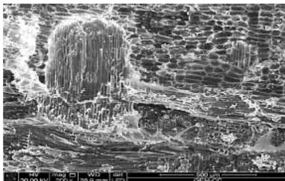
Fig.4: Shows SEM photomicrographs of archaeological wood in the mask (Mag. 200X, bar=500 $\mu$ m), loss of parts of the structure of wood as well as the presence of consolidants on the surface.
