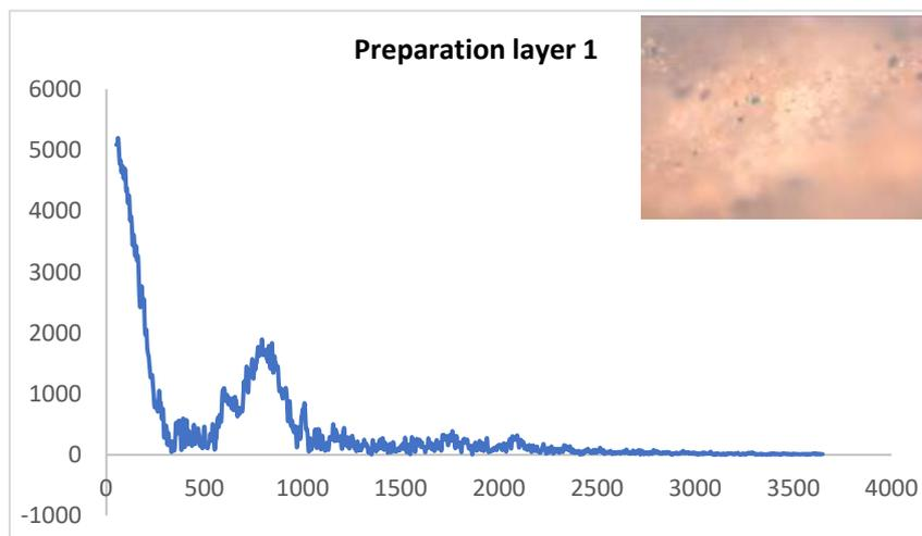
Fig 6. The sample of preparation layer showed the presence of calcite and clay minerals and a percentage of animal glue
