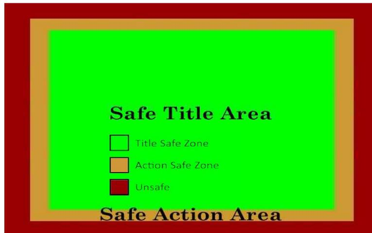
Fig.7 shows the safety zone in the TV scan
