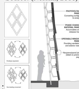
Fig. 27 – S.C.A.L.E.S. building envelope & adaptation mechanism
