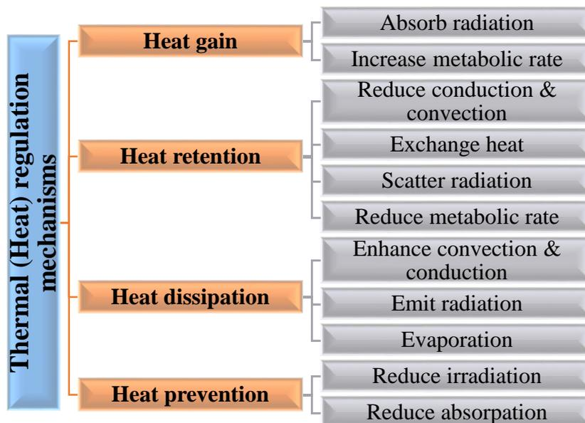
Fig. 2 – Thermal regulation mechanisms (functions & processes).
