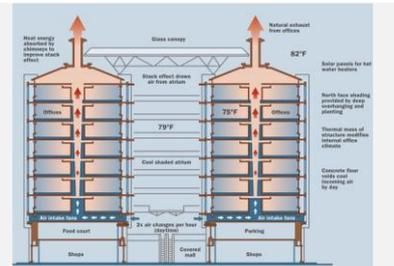
Fig. 17- Eastgate center section
