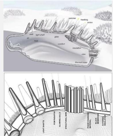
Fig. 36 – Proto Project envelope (structure & details)
