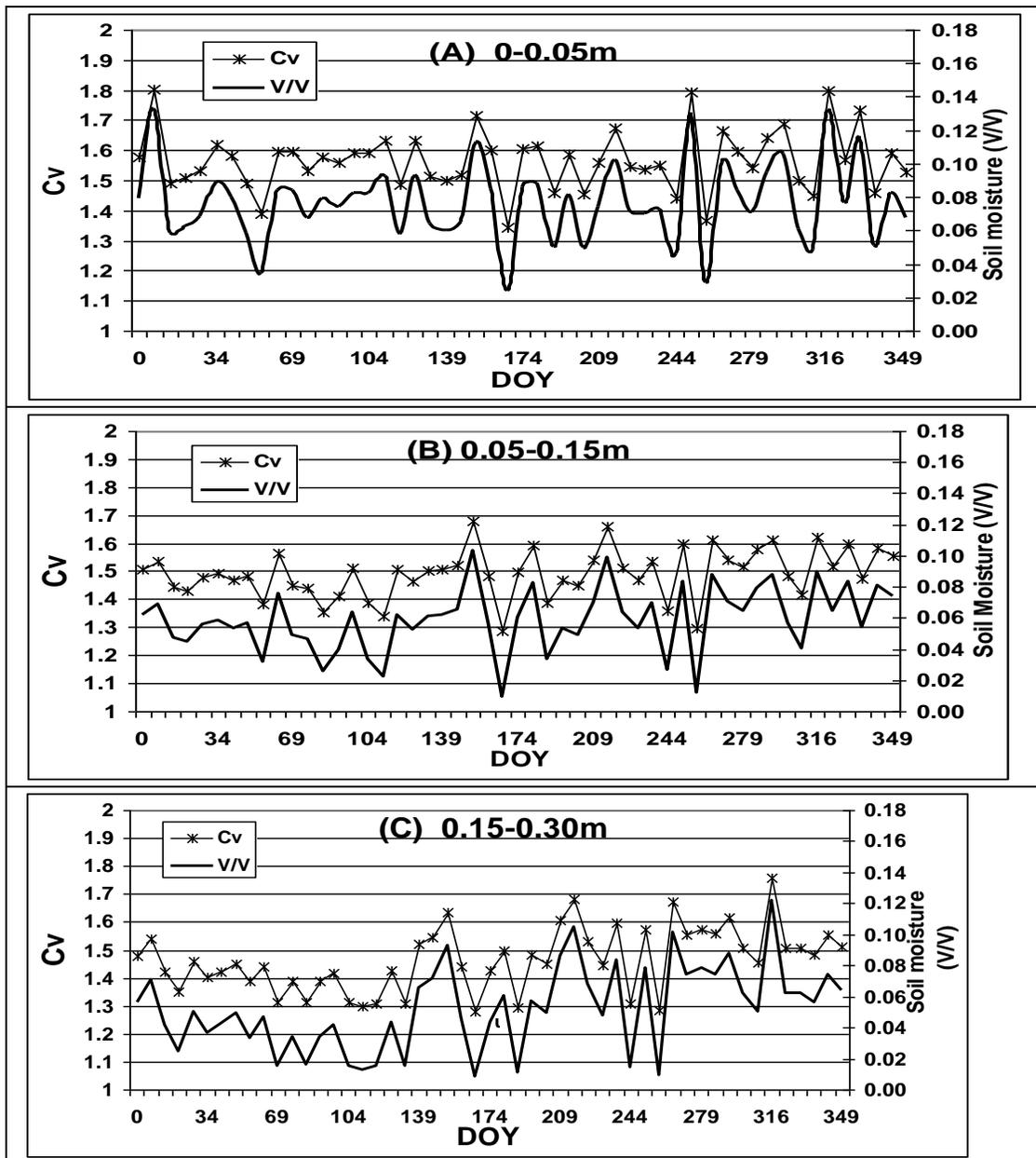
Fig.(1):Soil volumetric heat capacity (CV) ( $\text{MJm}^{-3}\text{c}^{-1}$ ) and volumetric moisture content (v/v) ( $\text{m}^3\text{m}^{-3}$ ) of the three soil depths (A,B and C), (DOY=Day of Year).
