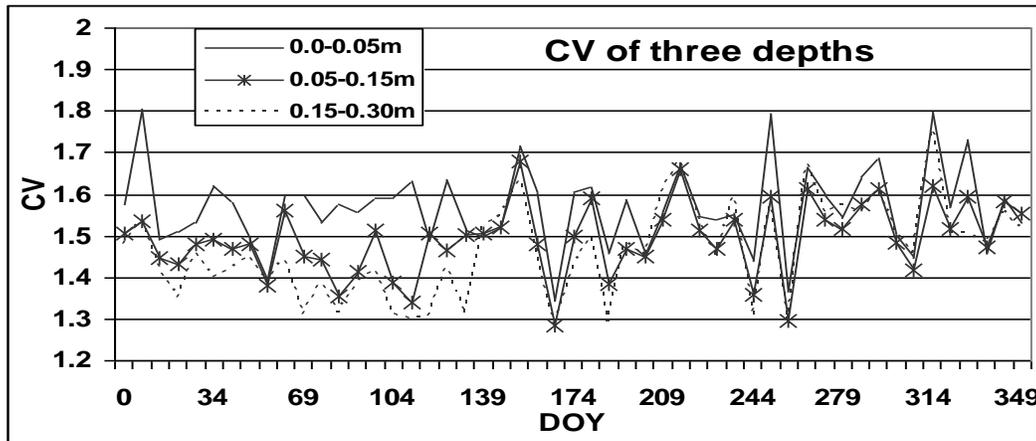
Fig. (2): Soil volumetric heat capacity ( $\text{MJm}^{-3}\text{c}^{-1}$ ) for three depths at 51 observations, (DOY = Day Of Year).
