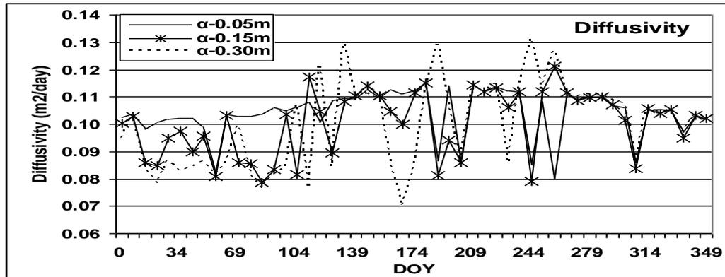
Fig. (6): Soil thermal diffusivity ( $\text{m}^2\text{day}^{-1}$ ) for three depths at 51 observation for three soil depths (DOY = Day Of Year).
