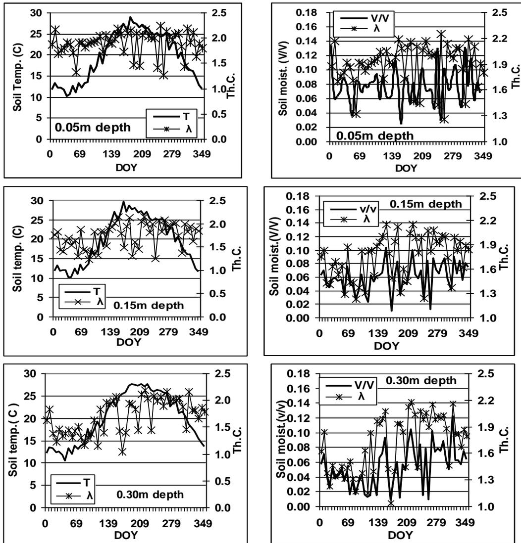
Fig. (3): Thermal conductivity (Th.C.) affected by soil temperature ( $^{\circ}\text{C}$ ) and soil moisture content ( $\text{m}^3/\text{m}^3$ ) through 51 observations at three depths (DOY=Day Of Year).
