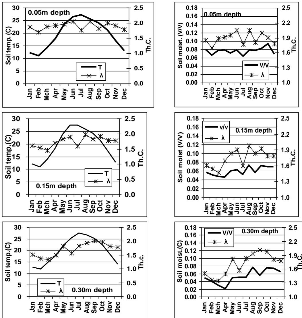
Fig. (4): Thermal conductivity (Th.C.) ( $Jm^{-1}s^{-1}c^{-1}$ ) (affected by soil temperature  $^{\circ}C$ ) and soil moisture content ( $m^3/m^3$ ) through Twelve months from January to December at three depths (DOY=Day Of Year).
