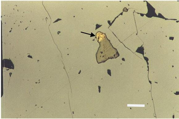
**Fig 10.** Composite Gold at the contact with sphalerite inside pyrite, Hammash gold mine, bare scale 20  $\mu\text{m}$ .
