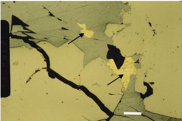
**Fig.9.** Gold associating galena inside pyrite, Abu Marawat gold mine, bare scale 20  $\mu\text{m}$ .
