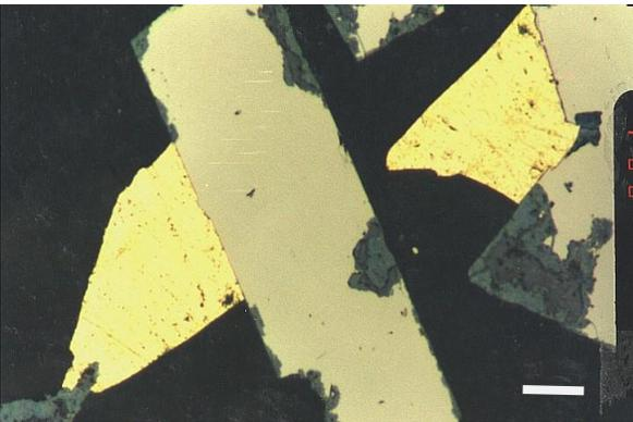
**Fig. 11.** Pure gold at the outer part of euhedral pyrite which reveals supergene alteration, Atud gold mine, bare scale 20  $\mu\text{m}$ .
