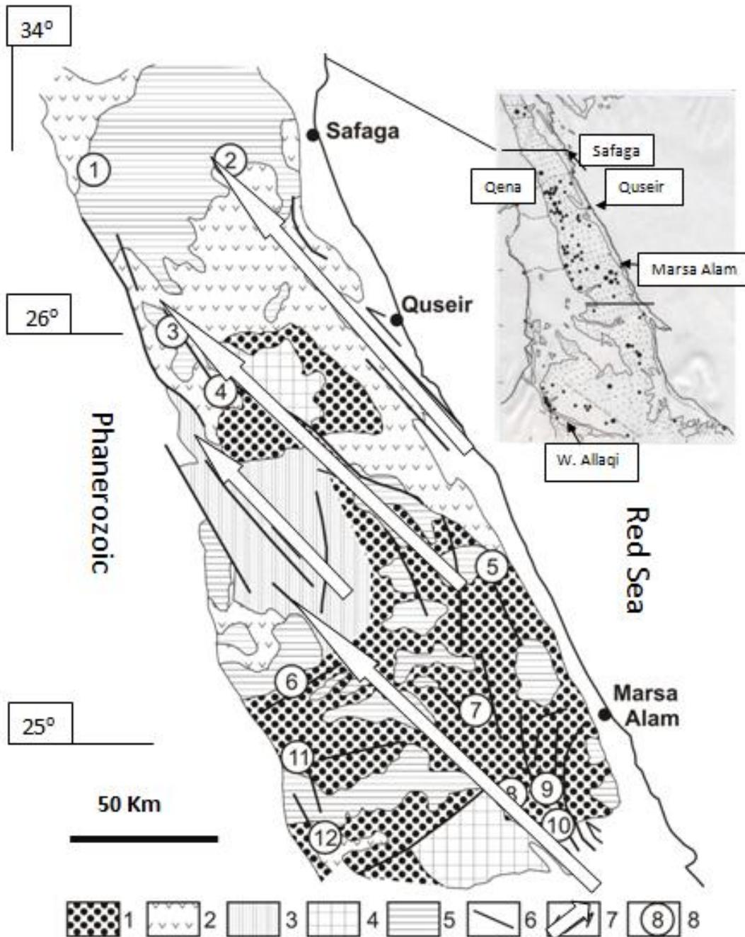
**Fig. 1.** Metallotect map of the Eastern Desert showing different rock assemblages and related gold occurrences, (compiled from <sup>[4,5]</sup>).
