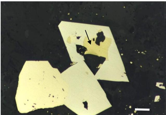
**Fig.5.** Gold (yellow) in arsenopyrite. Reflected light, Atalla gold mine, bare scale 20 µm.
