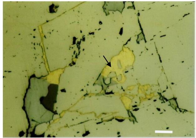
**Fig.6.** Gold (yellow) in micro fissures in pyrite, associating galena (gray) and sphalerite (dark gray) Reflected light, El Fawakhir gold mine, bare scale 20µm.
