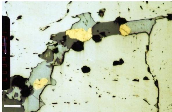
**Fig. 18.** Refract gold (yellow) and galena (light grey) and sphalerite (dark grey) cut through pyrite. Gold shows various reflectivities due to admixing elements. Um Ud, bare scale 20 μm.
