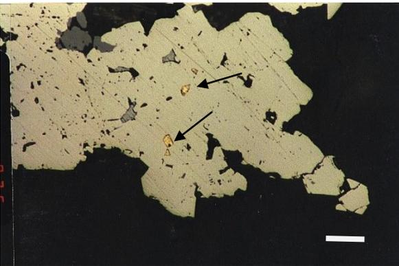
**Fig 13.** Very fine gold blebs inside pyrite with sphaerite micro-relicts. El Sid gold mine, bare scale 20  $\mu\text{m}$ .
