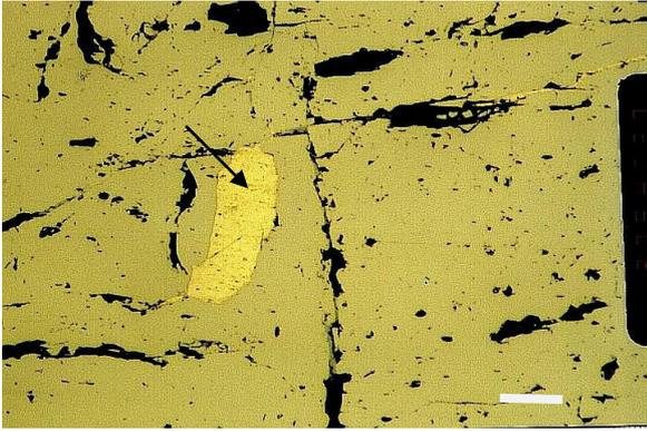
**Fig.7.** Pure Gold defused inside pyrite, gold hair inside very fine fractures, Hangaliya gold mine, bare scale 20  $\mu\text{m}$ .
