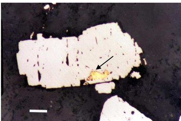
**Fig.14.** Native refract gold inside pyrite show micro-fracture in quartz, El Sukkary gold mine, bare scale 20  $\mu\text{m}$ .
