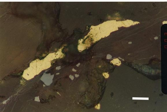
**Fig. 19.** Free mill gold inside sheared quartz with relicts of jarosite and anatase Um Garayat SED, bare scale 20 μm.
