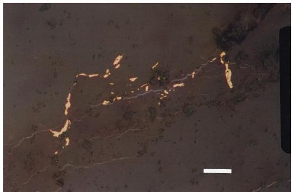
**Fig. 20.** Free mill native gold inside microfracture in quartz Um El Tuyor mine, SED, bare scale 20 μm.
