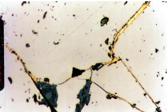
**Fig. 17.** Refract gold hairs (2- 5 microns thick) diffused along pyrite contacts, Umm Russ gold mine.
