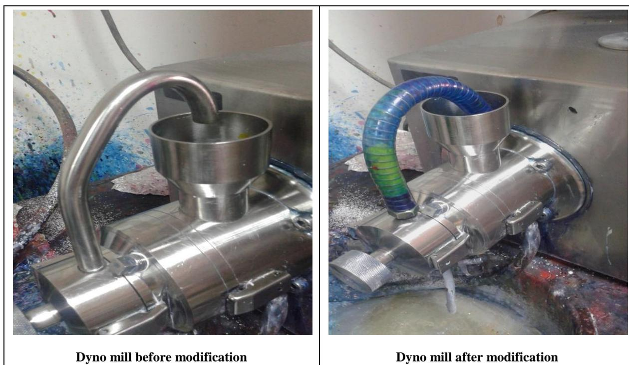
**Fig. 2:** Dyno mill (mini motor mill) before and after modification by flexible hose.
