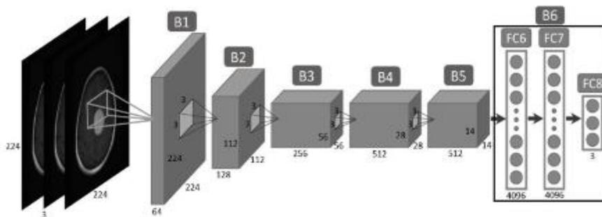
**Figure 4:** Block diagram of classification of MR brain images.
