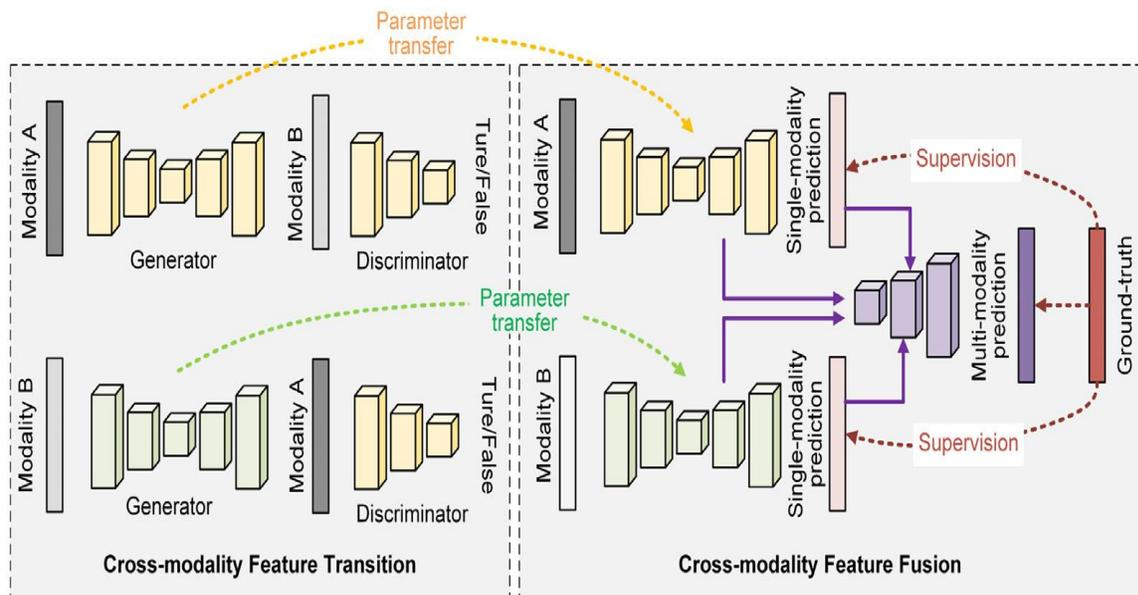
**Figure 5:** Block diagram of the brain tumor detection.
