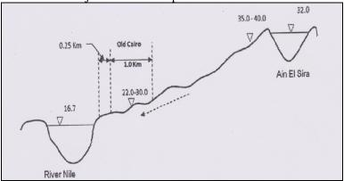
Figure 7- Sketch showing slopes and flow of untreated water
