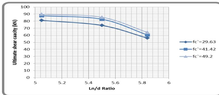
**Fig. (20)** Effect of clear span to the effective depth ratio ( $l_n/d$ ) on the ultimate shear strength for I-section.
