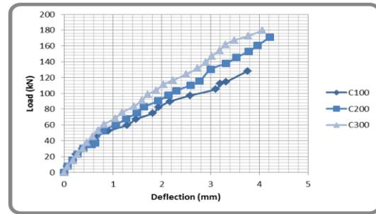
**Fig. (14):** Load –deflection curve for SCC I-section beams at compressive strength ( $f'_c$ ) =49.2 Mpa.
