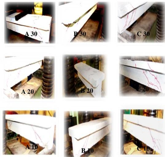
**Fig (21):** Crack pattern of SCCT-section beams.
