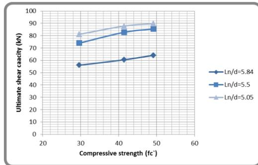
**Fig. (17):** Effect of compressive strength ( $f_c'$ ) for SCC I-section beams on the ultimate strength.
