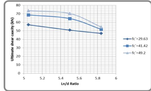
**Fig. (18):** Effect of clear span to the effective depth ratio ( $l_n/d$ ) on the ultimate shear strength for rectangular section.
