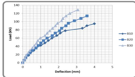
**Fig. (10):** Load –deflection curve for SCC T-section beams at compressive strength ( $f'_c$ ) =41.42 Mpa.
