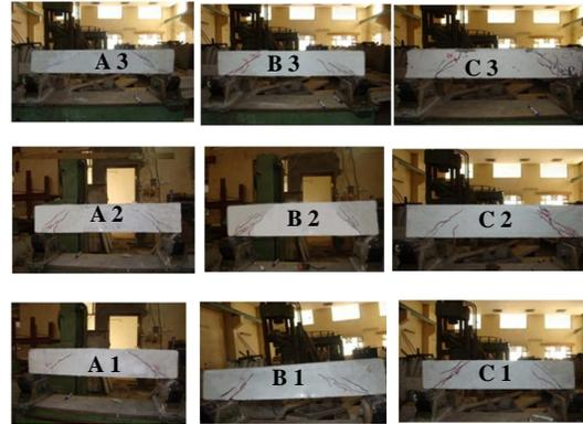
**Fig (20):** Crack pattern of SCC Rectangular beams.
