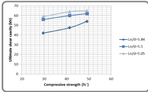
**Fig. (16):** Effect of compressive strength ( $f_c'$ ) for SCC T-section beams on the ultimate shear strength.
