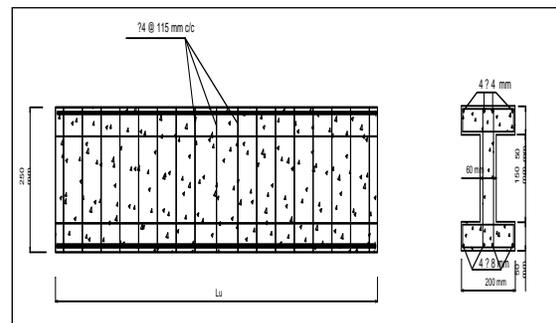
**Fig. (3):** Details of I-section all dimensions in mm.
