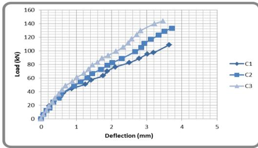
**Fig. (8):** Load –deflection curve for SCC rectangular beams at compressive strength ( $f'_c$ ) =49.2 Mpa.
