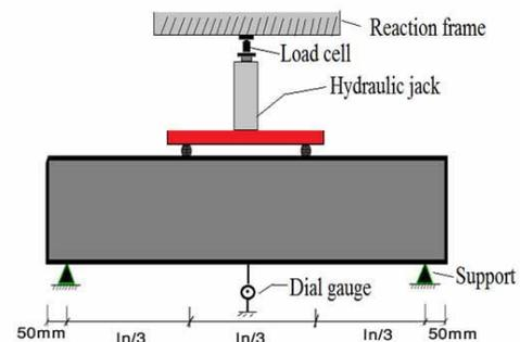
**Fig. (4):** Schematic diagram of test set-up.
