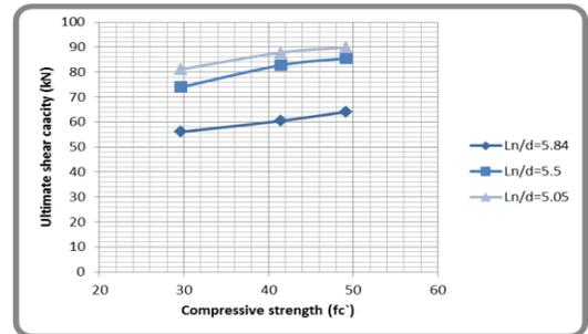
**Fig. (15):** Effect of compressive strength ( $f'_c$ ) for SCC rectangular beams on the ultimate strength.
