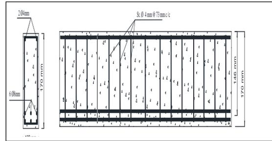
**Fig. (1):** Details of rectangular section all dimensions in mm.
