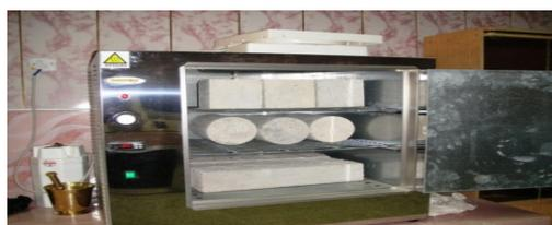
**Plate (1):** Layout of the specimens in oven.
