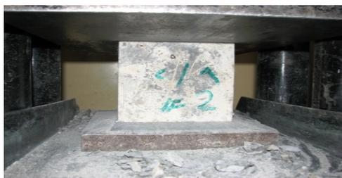
**Plate (2):** Testing Cubes Samples using Compression Machine.
