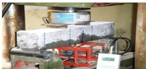
**Plate (3):** Testing Prisms Samples using Universal machine with capacity of 2000 kN.
