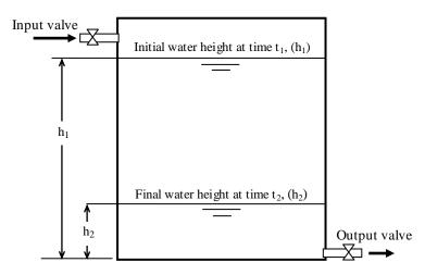
Fig. (1): Schematic of house reservoir
